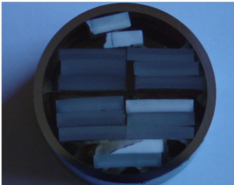
Figure 3.6: Sintered diffusion couples mounted in epoxy and polished to allow EMP measurements.
