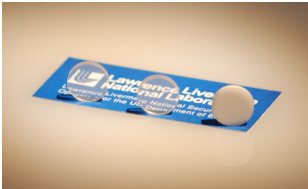
Figure 5.5: Effects of hot isostatic press treatment. Left: 1750 °C for 4 h at 200 MPa. Center: 1650 °C for 4 h at 200 MPa. Right: as-sintered.
