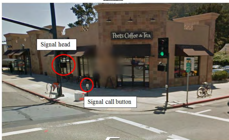
Figure 27. Example of “Pedestrian Signal Head” and “Pedestrian Signal Button”
