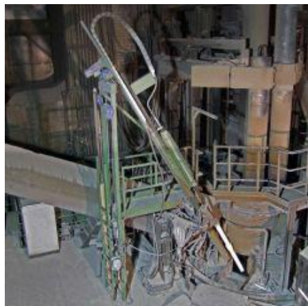
Figure 30. Photo of the device to measure steel temperature in EAF (BFI 2012)
