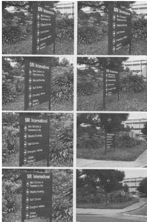
Figure 1.2: Suppose Z_{avg} is the average distance of an object from the camera and d_{avg} is the average width of the object (measured along the optical axis of the camera). As a rule of thumb, the orthographic camera model is reasonable to use when Z_{avg} \geq 10d_{avg} . In the figure above from Faugeras and Luong (2004), on the right, we see a scene containing a rectangular sign viewed by a projective camera as the photographer moves farther away from the sign. On the left, the portion of each image containing the sign is cropped and re-sized so that the sign occupies approximately the same area. It is evident as the camera moves farther away that the perspective effects diminish. In particular, the vanishing point for the parallel lines on the top and bottom of the sign moves increasingly close to infinity. Alfred Hitchcock pioneered the use of this effect (the so-called “Hitchcock zoom”) in the movie Vertigo .
