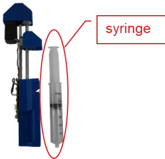
Figure 32 Print head for hexaferrite-SU8 composite; the syringe can be purchased separately
