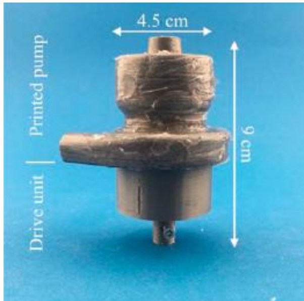
Figure 60 Fully printed pump with drive unit after removal of support material (no magnets visible, coated with silicone)[56] .
