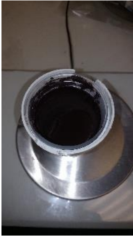
Figure 64 Mixture of dissolved ABS and barium hexaferrite particles.
