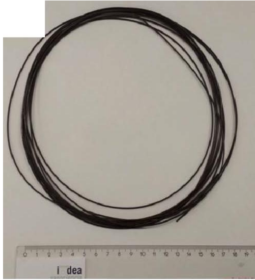
Figure 66 SrM and ethylene ethyl acrylate (EEA) polymer extruded filament[11]; filaments similar to this was made with BaM and ABS/PLA
