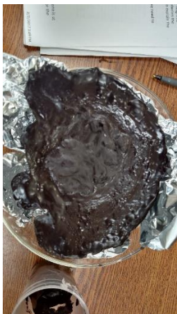
Figure 65 Dried mixture of ABS and hexaferrite particles.
