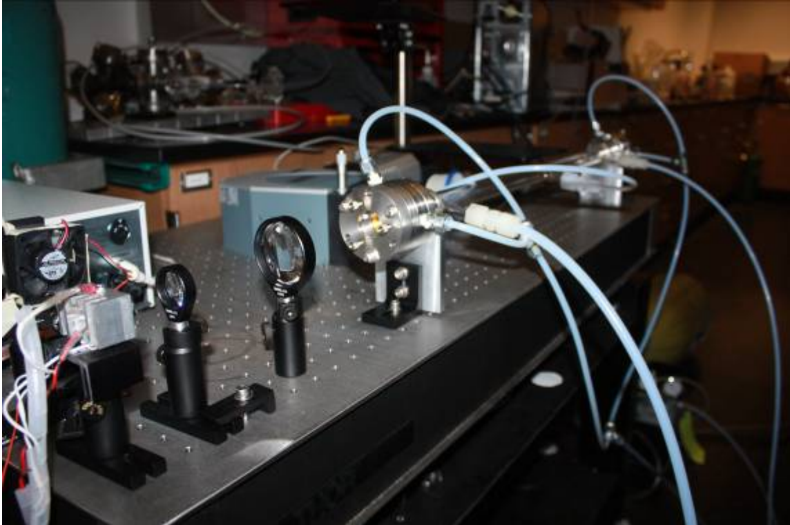
Figure 5.2b: Close up view of the BBCEAS instrument. The LED is mounted on a thermally controlled aluminum block. Two lenses are used to focus the light into the front mirror of the cavity.
