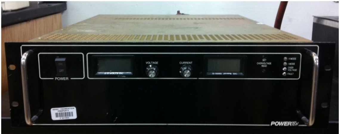
Figure 4.7 Power Ten P63- 51000 1000A, 5V power supply
