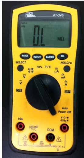
Figure 4.13 Commercially available multi-meter used in the testing of thermocouple conductivity with the specimens
