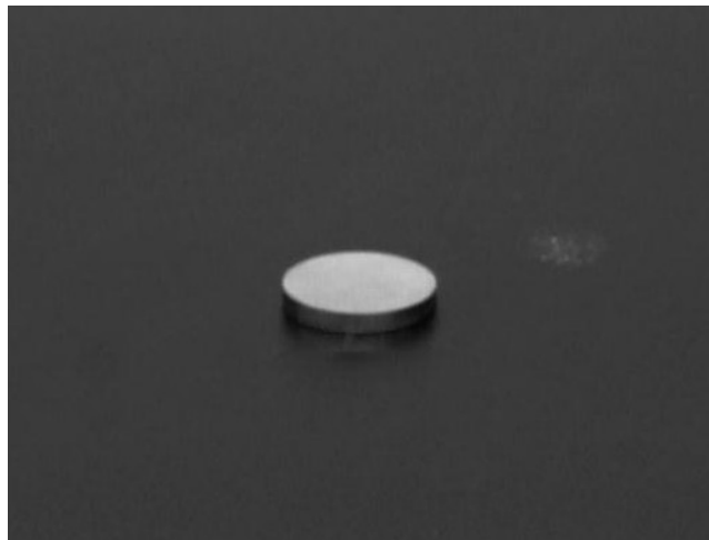
Figure 4.5 Nickel powder compact (12.1mm diameter, 1mm thick)
