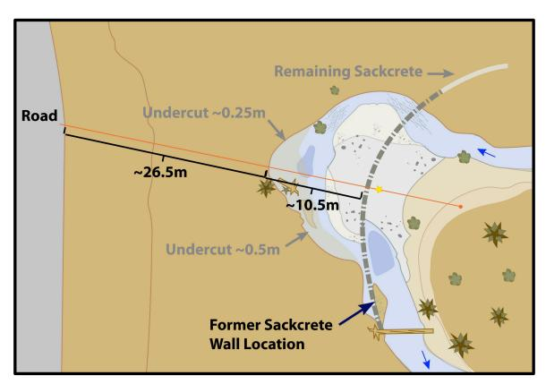
FIGURE 4: Sackcrete Bend current plan view
