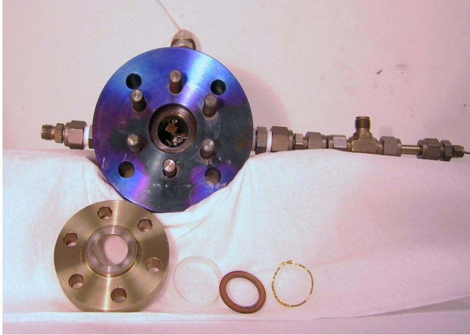
Figure 1. A photo of titanium autoclave parts
