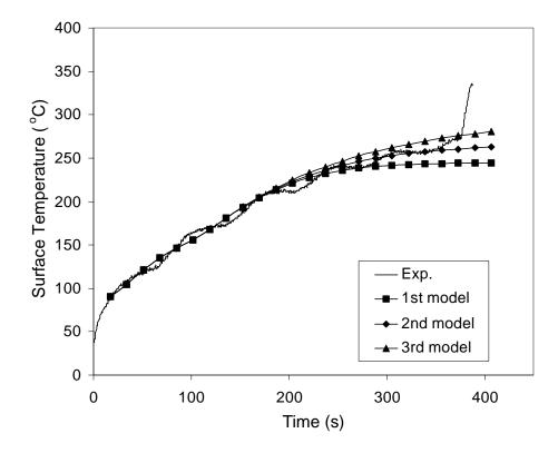
Figure 7. Predicted variation with time of the sample surface temperature for the three models
