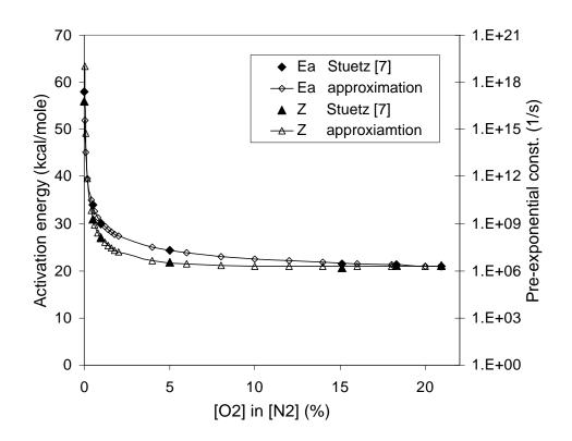
Figure 5. Pre-exponential constant and activation energy as a function of oxygen concentration
