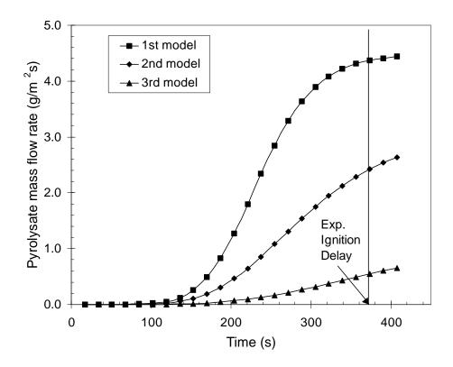
Figure 6. Predicted oxygen concentration effect on the pyrolysate mass flow rate for the three models of oxygen distribution
