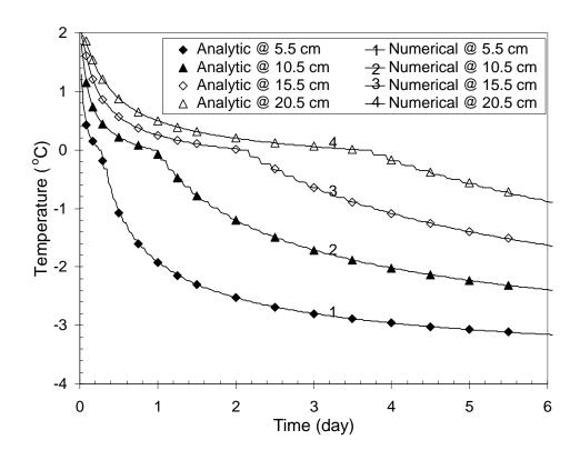
Figure 3. Comparison of numerical and analytic temperature history at several positions for the classical Stefan problem
