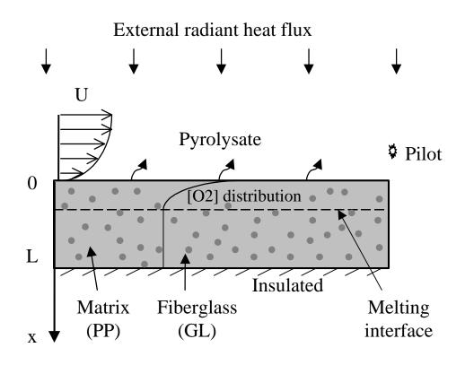
Figure 4. Schematic of the pyrolysis and ignition of a composite
