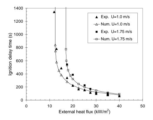
Figure 8. Predicted external heat flux effect on ignition delay for two flow velocities using the second model
