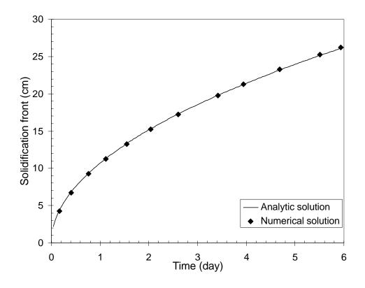
Figure 2. Position of the phase change interface vs. time for the classical Stefan problem
