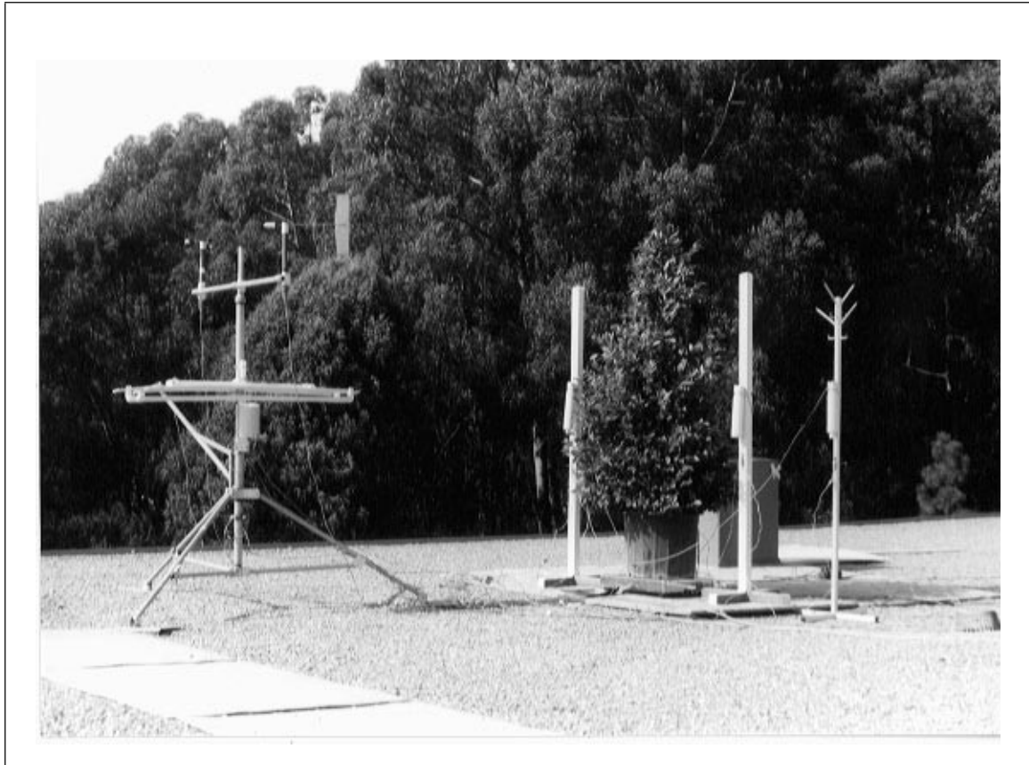
Figure 6-1. Weather station and potted tree on third-story building roof in Berkeley, CA. A linear array of air temperature sensors surrounds the tree. A shaded assembly of PVC piping, used to join the air temperature sensors to a common air source for mutual calibration, is mounted halfway up the weather tower.
