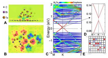
**Fig. 4. Theoretical calculations. (A** and **B)** Side and top views of the atomic structure and charge-density difference of  $Bi_2Te_3/g$ raphene. Red and blue colors indicate charge depletion and accumulation, respectively. (**C** and **D**) Band structure of  $Bi_2Te_3/g$  graphene. (**E**) n-field configuration with red solid, blue hollow circles, and blank boxes denoting n = -1, 1, and 0, respectively. Summing the n-fields over half of the torus yields a nontrivial  $Z_2$  invariant.
