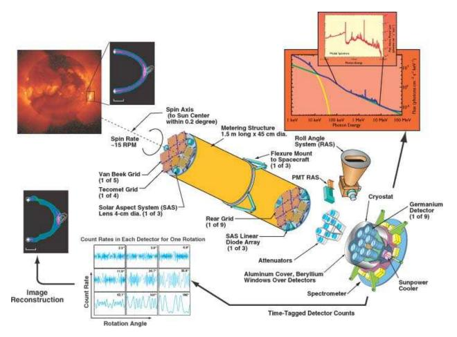
Figure 3.1: Illustration showing the components and capabilities of the *RHESSI* instrument; image from Lin et al. (2002). The imaging system consists of nine pairs of grids separated by 1.55 m and works by modulating source flux as the spacecraft spins. This Fourier-based method of imaging can resolve sources down to 2.3 arcseconds. The detector system is composed of nine identical coaxial high-purity germanium detectors, offering good energy resolution and sensitivity up to 17 MeV.
