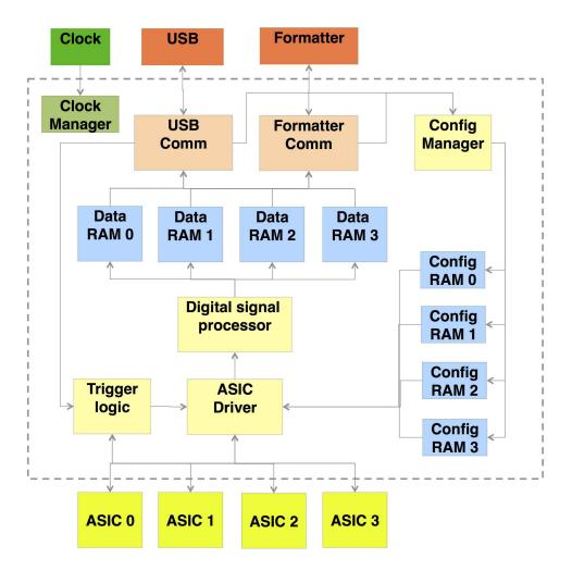
Figure 8.14: Block diagram of the FPGA functions, including SRAM memory, communication, timing, and processing modules. For simplicity, several FPGA modules are left out of the diagram and several buses are condensed into single lines. Boxes outside the dashed line are external to the FPGA. Each detector has a dedicated FPGA, which is interrogated independently by the formatter.
