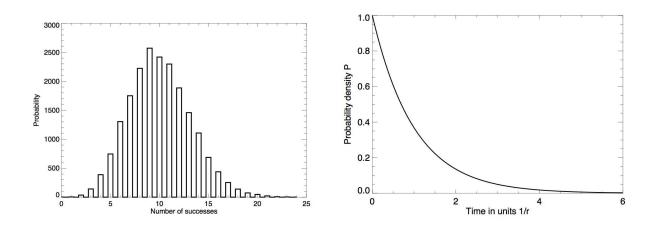
Figure 8.7: (Left) A Poisson probability distribution for 10 mean successes. (Right) Poissonian distribution of waiting times between successive events, with waiting times in units of the inverse count rate r, and with the distribution normalized to r.
