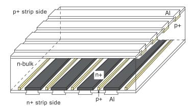
Figure 8.5: Diagram of a double-sided strip detector. Holes and electrons are collected at strips on the p- and n-sides that are oriented orthogonally to each other so that a two-dimensional image can be obtained. Each strip acts as an individual p-n junction. The "p-stops" improve charge collection on the n-side and will be discussed in Section 8.2.1. Figure from Takeda et al. (2008).
