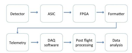
Figure 8.11: Flowchart for *FOXSI* data handling. After data is measured, digitized, and read out from each detector by four ASICs, a FPGA performs minor processing and data reduction. The formatter FPGA then packages all the detector data into a telemetry stream, which is transmitted to a ground station at White Sands and fed into the *FOXSI* DAQ software for live monitoring of flight data. After the flight, data is processed into Level 1 products and analyzed.
