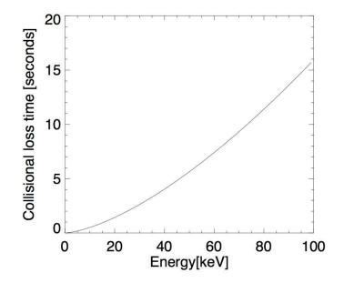
Figure 5.10: The collisional stopping time for energetic electrons in a plasma of density  $5 \times 10^9$  cm<sup>-3</sup>.
