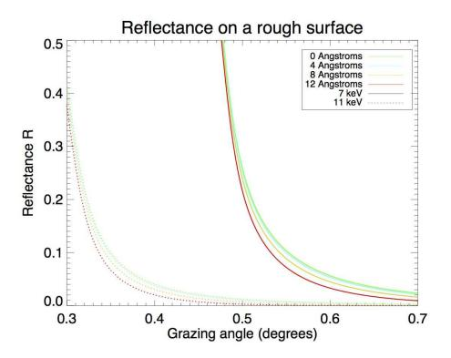
Figure 7.3: X-ray reflectivity for a thin nickel layer with surface roughness included, for 7 keV photons (solid line) and 11 keV photons (dashed line). Surface roughnesses range from 0 to  $12\mathring{A}$  RMS. Calculations were done using the IMB software (Windt 1998).
