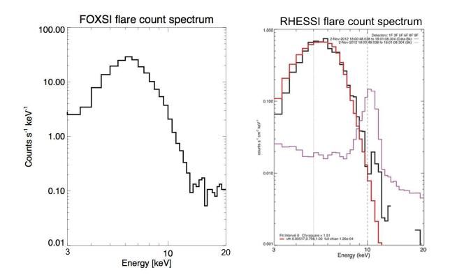
Figure 9.5: Microflare count spectra from (left) the *FOXSI* sounding rocket and (right) the *RHESSI* spacecraft. *RHESSI* spectral fitting reveal that the flare had a temperature of 9 MK and an emission measure of  $5 \times 10^{46}$  cm<sup>-3</sup>.
