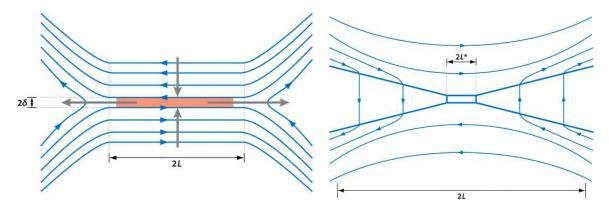
Figure 2.1: (Left) Diagram of the Sweet-Parker model of reconnection, including a thin, long current sheet, inflow (vertical arrows) and outflow (horizontal arrows). (Right) The Petschek model, in which the diffusive region has a finite length and width. Not all particles make it into the diffusive region; many instead are redirected at the standing shocks. Both figures are from Zweibel & Yamada (2009).
