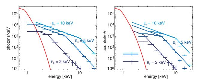
Figure 6.6: Simulations of spectra for nonthermal (blue) and 2 MK thermal (red) X-rays from quiet-Sun network flares. On the left, simulated photon flux is shown for various values of the cutoff energy  $E_0$ , with a fixed power-law index of 5 above and 1.7 below the break. In the righthand plot, data points and error bars show the expected *FOXSI* count spectra. Both plots are from (Krucker et al. 2011b)
