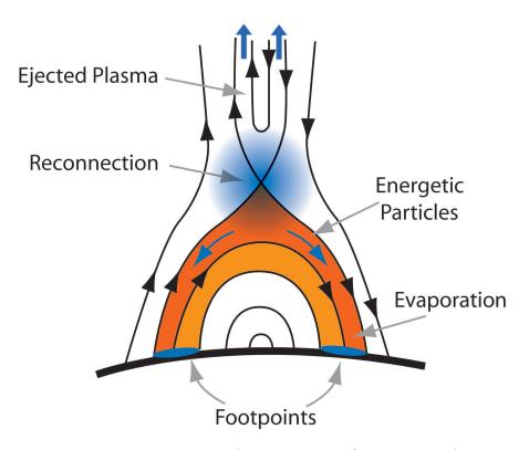
Figure 2.3: Two-dimensional diagram of the standard flare model. A rising plasmoid (not shown) instigates reconnection with the overlying coronal field, producing the magnetic field drawn here. Particles are accelerated in the shaded central region; energized electrons can then stream down the flare loops (orange), or escape upward into interplanetary space. Image is from Christe (2007), based on Sturrock (1966).
