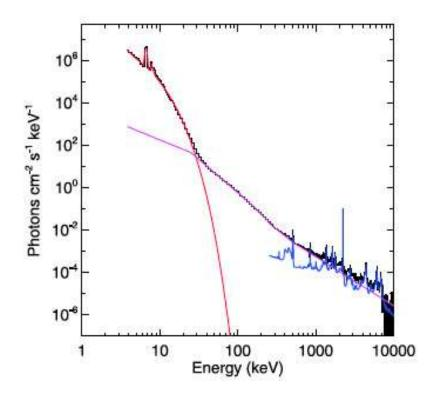
Figure 2.7: A sample *RHESSI* X-ray spectrum from the 2002 July 23 class X4.8 solar flare, showing thermal (red) and nonthermal (pink) components, as well as gamma ray lines from nuclear contributions (blue). Image is from Lin (2011).
