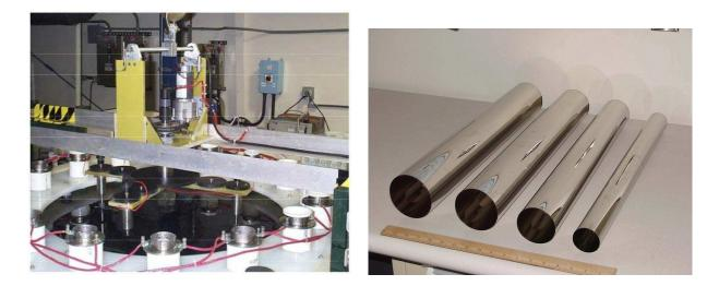
Figure 7.7: (Left) An electroforming bath at MSFC for plating ENR optics. (Right) Several *HERO* shells of various diameters. Both images are from Ramsey et al. (2004).
