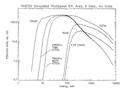
Figure 3.5: Effective area for the *RHESSI* detectors for photopeak absorption, image from Smith et al. (2002). The effective area is shown for the front and rear segments separately and for multiple attenuator states. The total area includes the front- and rear-segments with no attenuators and the F/R coincidence curve shows the area for events measured in both front and rear segments.
