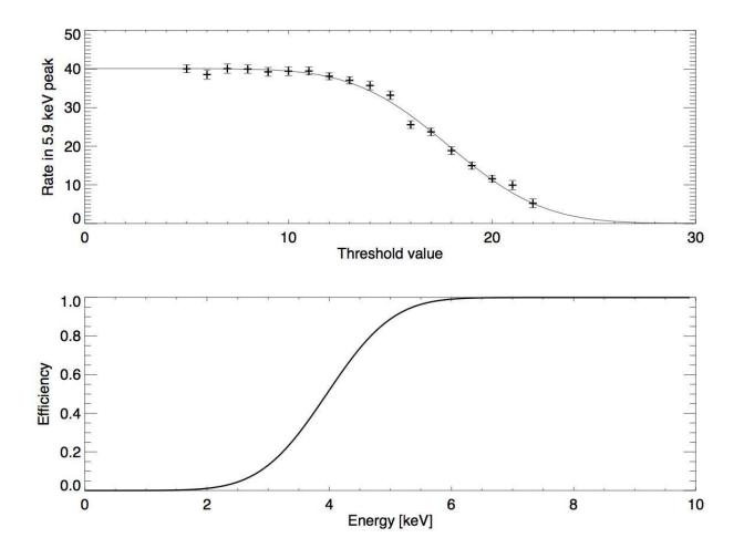
Figure 8.20: Example of the measurement of the detector efficiency near the low energy threshold. (Top) Measured count rates in the Fe-55 5.9 keV peak, with the best fit curve overplotted. Error bars are statistical uncertainties. (Bottom) The corresponding efficiency for a threshold value of 12; this is the value chosen for flight. This measurement is for one p-side ASIC of detector 101.
