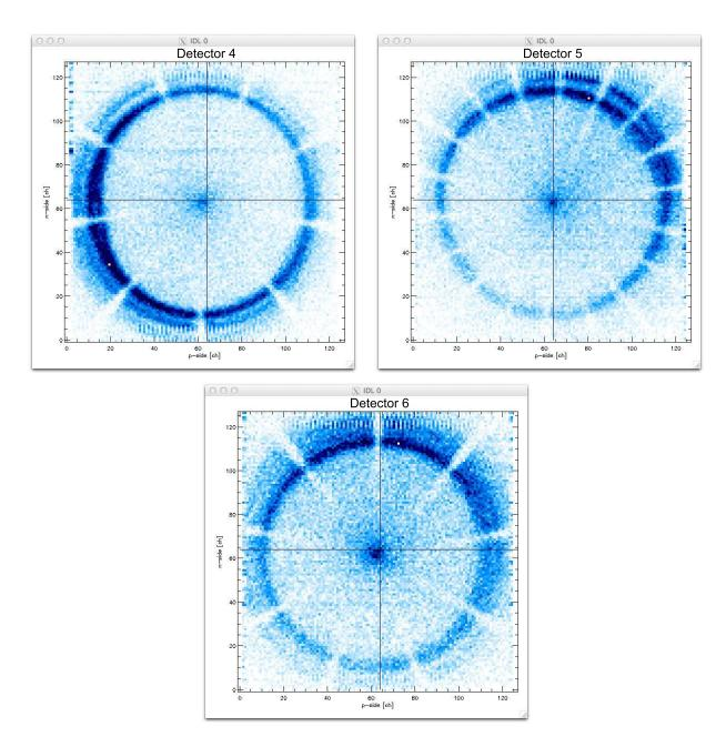
Figure C.2: X-ray images for detectors 4–6. In the detector 5 (upper right) image, more spokes (corresponding to slats in the spider supports) are apparent because of a phase offset between spider supports on either side of the module.
