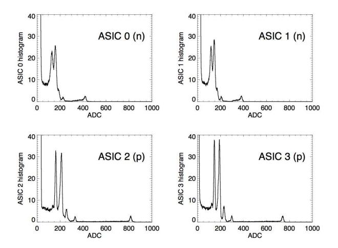
Figure 8.17: Uncalibrated Am-241 spectra taken with detector 101, in raw ADC values with the common-mode values subtracted. Spectra for each ASIC is shown; the relatively poor performance of the n-side as compared to the p-side is evident.
