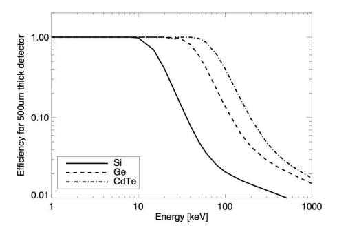
Figure 8.6: Efficiency as a function of X-ray energy for a 500  $\mu$ m thick detector. Silicon, the lowest-Z material considered here, has appreciable efficiency only up to tens of keV. For higher energy HXR and gamma-ray studies, higher-Z materials like germanium and cadmium telluride must be used.
