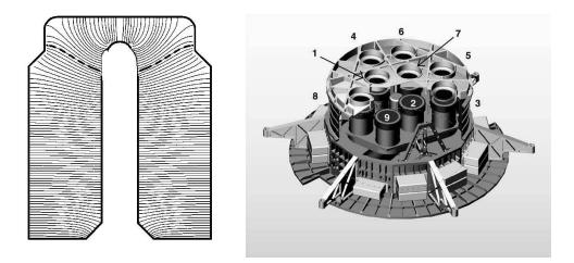
Figure 3.4: The *RHESSI* detector system, images from Smith et al. (2002). (Left) Crosssection of a single coaxial Ge detector, showing example field lines and segmentation. (Right) Model of the full set of nine Ge detectors. Each detector has a corresponding subcollimator in the imaging system.
