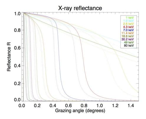
Figure 7.2: Reflectance of X-rays from 1 to 80 keV vs grazing incidence angle for a 0.25 mm thick layer of nickel (solid lines) or iridium (dashed lines), computed using the IMD package for IDL (Windt 1998). The interface was modeled as a step function with no roughness.
