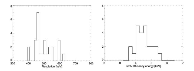
Figure 8.19: Histograms of (left) the energy resolution at the 13.9 keV Am-241 line and (right) the threshold energy at which the system is 50% efficient for all detectors with the *FOXSI* VATA451 ASIC. The values were measured separately for each p-side ASIC. Some detectors were read out with a different iteration of this ASIC, the VATA450; these detectors were not used for flight and are not included in this histogram.
