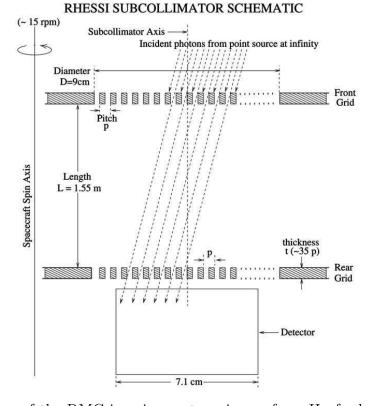
Figure 3.2: Diagram of the RMC imaging system, image from Hurford et al. (2002). Each subcollimator has two identical-pitch grids widely spaced apart. Transmission of X-ray flux through the grids depends on the orientation of the source with respect to the grids. As the spacecraft rotates, this orientation changes and the transmitted flux is modulated in a way that captures two-dimensional spatial information.
