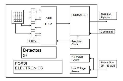
Figure 8.12: Block diagram of the *FOXSI* electronics package. Each of the 7 detectors has 4 R/O ASICs and a dedicated FPGA. Data from each FPGA is collected by a formatter FPGA (encoder) and packaged into a data packet inserted into the telemetry stream. Power, telemetry, and uplink commanding are provided by the NASA Sounding Rocket Operations (NSROC) team.
