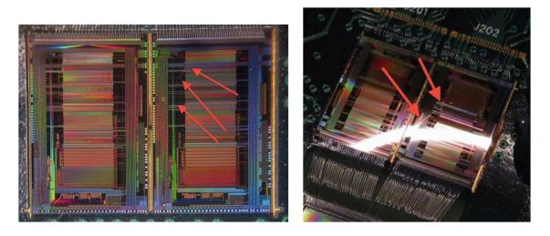
Figure 8.16: Photographs of selected ASICs with visible fractures after the cooling accident. Differential thermal expansion cracked the chips, rendering them inoperable.
