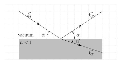
Figure 7.1: Ray-tracing diagram demonstrating Snell's law.  $\vec{k_I}$ ,  $\vec{k_R}$ , and  $\vec{k_T}$  are the incident, reflected, and transmitted rays, respectively.
