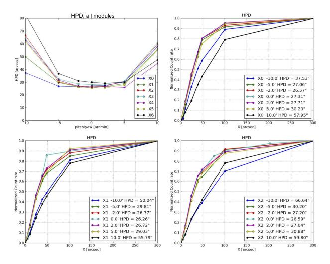
Figure A.1: The HPD was measured by taking data with various sized pinholes placed over a detector. The extrapolated pinhole size (in arcseconds) that encompasses half the flux measured by the largest pinhole is taken to be the HPD. The top left plot is a summary showing this measurement for all the optics modules (labeled X0–X6) for an on-axis and several off-axis configurations. Detailed plots showing the actual measurements for each module follow in this and the next figure.
