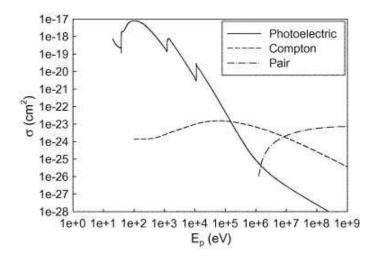
Figure 8.2: Cross sections of photon interactions in germanium. Up to  $\sim 100$  keV, photoabsorption is the most likely interaction. Results are similar for interactions in silicon. Figure from Gao et al. (2007).
