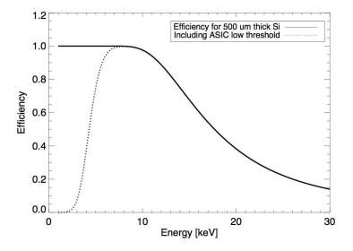
Figure 8.9: Efficiency of the *FOXSI* detectors for the X-ray energy range of interest. The dashed line includes the effect of the low-energy threshold (LET) of the VATA451 ASIC and is an averaged value from all of the ASICs used for flight. (Details of this measurement will be discussed later in this chapter.) Attenuation length data is from Henke et al. (1993).
