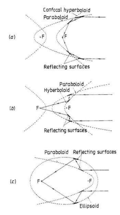
Figure 7.6: Wolter type I, II, and III geometries; from Aschenbach (1985).
