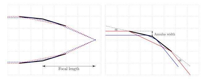
Figure 7.13: Ray diagram for a single Wolter-I mirror shell, with a closeup showing the annulus that is the collecting area for that mirror. In this drawing, the parabolic and hyperbolic shapes are approximated by straight lines.
