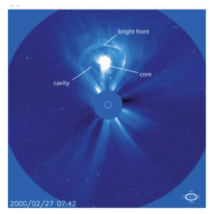
Figure 5.1: An example of a CME observation from the *Large Angle Spectrometric Corona*graph (LASCO) aboard SOHO. A coronagraph uses an occulting disk to block bright light from the solar disk, allowing faint reflected light from the corona to be measured. This example shows the typical bright front, dark cavity, and bright core often observed in CMEs. Image is from Riley & McComas (2009).
