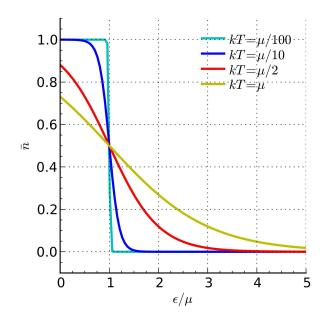
Figure 8.4: Occupancy of energy states in a Fermi distribution, for various temperatures.  $\mu$  is the Fermi energy. For  $kT \ll \mu$ , all states with energy  $\epsilon \ll \mu$  (i.e. valence band) are filled and all those with energy  $\epsilon \gg \mu$  (conduction band) are empty. As kT approaches the Fermi energy, thermal fluctuations allow more electrons into the conduction band.
