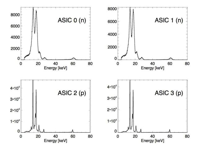
Figure 8.18: Calibrated Am-241 spectra for all ASICs of detector 101.
