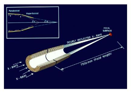
Figure 6.2: Schematic of a grazing-incidence focusing X-ray telescope. Incident photons undergo a double reflection before being focused. Typically, mirrors of different diameters are nested together to increase the effective area of the instrument. Image is from Ehle et al. (2001).
