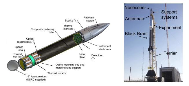
Figure 9.1: (Left) Schematic of the experimental section of the *FOXSI* payload. (Right) Photograph of the *FOXSI* rocket on the launch rail at White Sands. The experiment section is enclosed in a styrofoam box for temperature control. Non-flight equipment (liquid nitrogen, a cooling controller, and temperature sensor monitors) was located on the launch rail next to the experiment section. The two rocket stages include Black Brant and Terrier motors.
