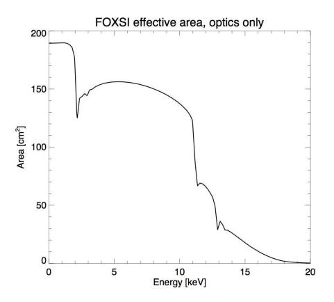
Figure 7.9: Theoretical effective area of the *FOXSI* optics, all shells and all modules combined.
