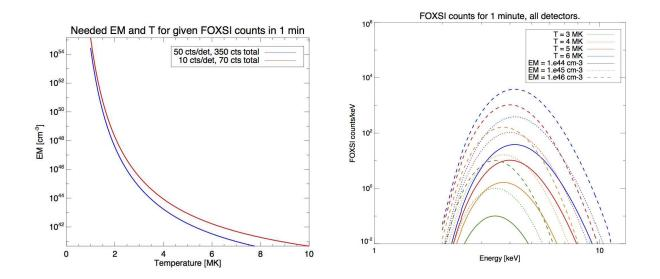
Figure 6.4: (Left) The parameter space of emission measure (EM) and temperature to which FOXSI is sensitive. Shown here are the values of the EM and temperature that would produce 350 (blue) or 70 (black) total counts in the FOXSI instrument in one minute. The higher the temperature, the lower the emission measured needed to produce this count rate. (Right) Simulated FOXSI counts for one minute for several emission measures and temperatures.
