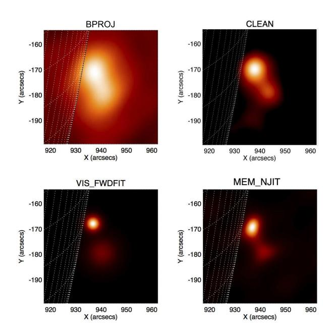
Figure 3.6: Comparison of images made using several standard RHESSI imaging algorithms, including (upper left) back projection, (upper right) Clean, (lower left) visibility forward-fit, and (lower right) Maximum Entropy Method images. The double nature of the source is observed clearly with the visibility-based routines (bottom row). All images are from the time interval 2003 August 21 15:16:15–15:18:00 UT, in the energy range 10–25 keV, and made using subcollimators 3–9.
