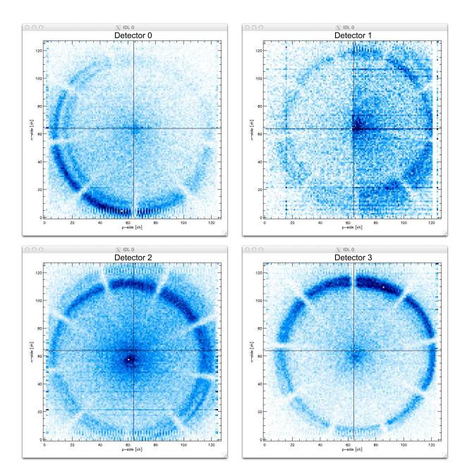
Figure C.1: X-ray images for detectors 0-3. Optic 0 (upper left) is the least well-aligned (2 arcmin), while most of the other optics are aligned to <1 arcmin. Problems with a readout ASIC result in poorer quality data for detector 1 (upper right).
