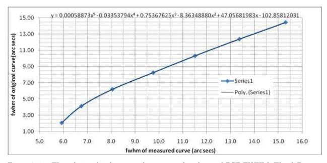
Figure 7.11: The relationship between the measured and actual PSF FWHM. The difference between the two is an effect of the large (50  $\mu$ m) pinhole used in the measurements.
