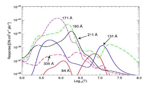
Figure 5.3: Temperature response of the six AIA filters sensitive to hot coronal plasma. Measurement in a single filter is insufficient to infer a temperature. By combining data from multiple filters, temperatures can be obtained. Note that the filters with best sensitivity to  $\sim 10$  MK plasma are 131 and 94 Å. Figure is from Lemen et al. (2012).
