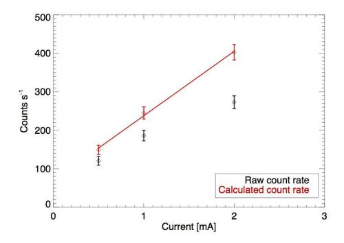
Figure 8.23: Count rates measured from a an X-ray generator 20 meters in front of the payload, with X-rays focused by the optics onto detector 6. Black data points are the raw measured count rates, with no livetime correction. Red data points are the rates reconstructed by fitting the livetime distribution. The red line shows a linear fit to the data.
