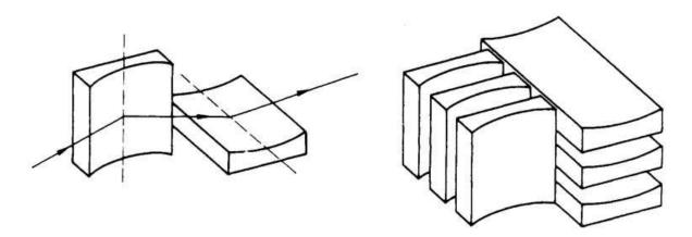
Figure 7.5: Schematic of a Kirkpatrick-Baez configuration; from Aschenbach (1985).
