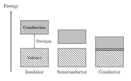
Figure 8.1: Energy bands for three types of solids (not to scale).
