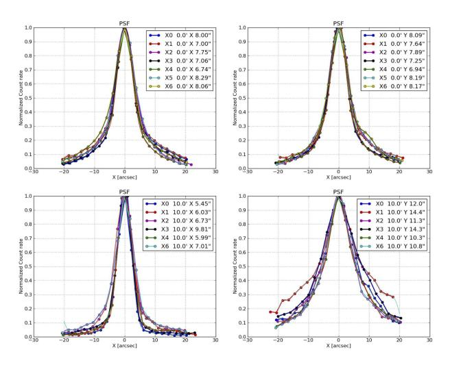
Figure A.3: The PSF was measured by stepping a single-pixel detector across the core of the focused X-ray image. This measurement was performed for an on-axis (top panels) and for one off-axis (10 arcminutes, bottom panels) position. The FWHM in both dimensions is shown for each module. The off-axis PSF is squeezed in the radial direction and elongated in the azimuthal direction, with respect to the center of the field of view.
