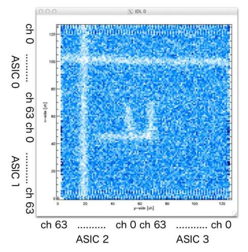
Figure 8.21: An image test for one of the first *FOXSI* detectors tested at SSL. The mask ('F' plus two lines) made by fine lines of solder is clearly visible. At the top and bottom of the image a checkered pattern indicates the locations of wirebonding pads, which alter the collection properties of the underlying detector volume (Ishikawa et al. 2011).
