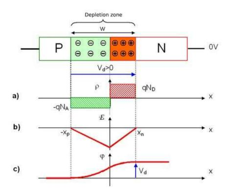
Figure 8.3: Sketch demonstrating the electrical properties surrounding a p-n junction. Even in the absence of an applied bias voltage there is a built-in potential and depletion region. Applying a reverse bias voltage (positive potential to the n-side) will increase the width of the depletion region. Image from Servagent (2007).
