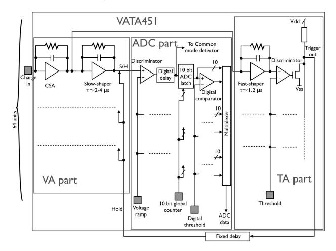
Figure 8.10: Block diagram of the VATA, showing the charge-sensitive amplifier, slow shaper and sampling circuitry (VA part), ADC, and fast shaper for triggering (TA part). Image from Ishikawa et al. (2011).
