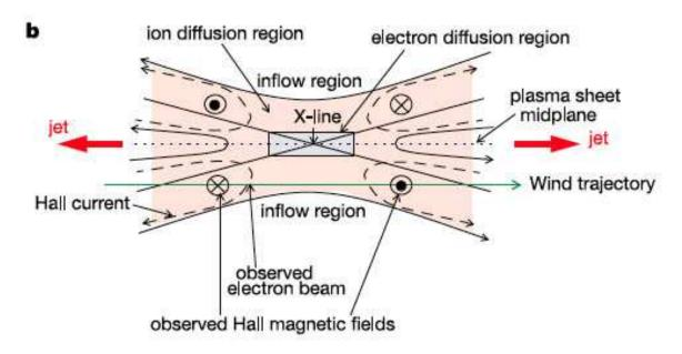
Figure 2.2: A diagram of collisionless Hall reconnection. On scales smaller than the ion gyroradius, ions are not bound to field lines and Hall effects become important. The ion diffusion region is larger than the electron diffusion region, allowing for reconnection on appropriate time scales. This picture has been well-validated in the Earth's magnetotail and could also be applicable to solar flares. Figure is from Lin (2011).
