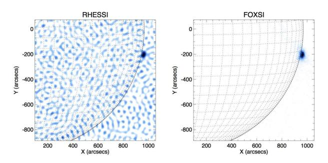
Figure 9.4: A comparison of (left) a *RHESSI* Clean image and (right) a *FOXSI* image of the B2.7 flare observing during *FOXSI*'s flight. Each image is scaled to the maximum intensity for that image. The *RHESSI* image shows artifacts that reduce the dynamic range of the instrument even far from the bright source. The *FOXSI* image is clean of such artifacts, enabling a much higher dynamic range.
