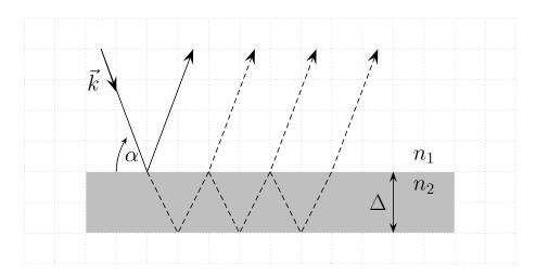
Figure 7.4: Diagram showing paths for a wave entering a thin slab. In addition to a simple reflection (solid line), the wave could reflect once or more within the slab (dashed lines).
