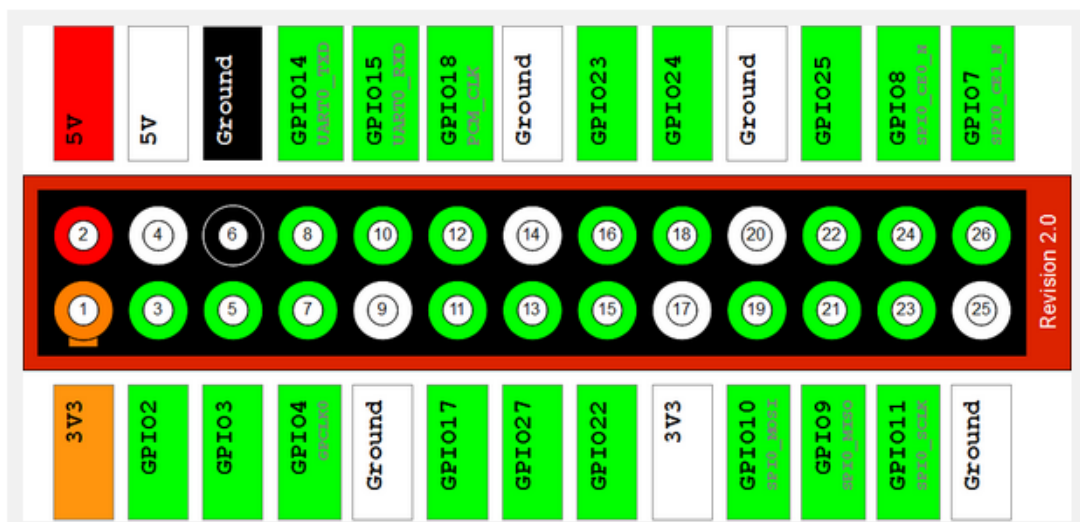
Fig. 3. 8 Raspberry Pi GPIO Layout – Revision 2. From reference 36
