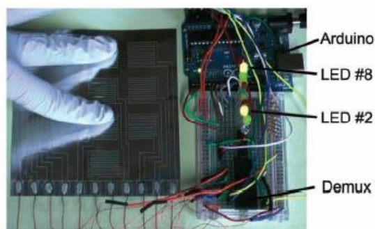
Fig. 2. 5 Touch pad with 10 keys that produced measurable changes in capacitance (a) constructed keypad and circuit, (b) measurement results. Reproduced from Reference Citation 27 with permission of The John Wiley and Sons.
