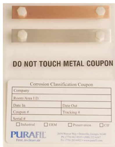
Figure 1 – Unexposed Corrosion Classification Coupon Containing Copper and Silver Metal Strips
