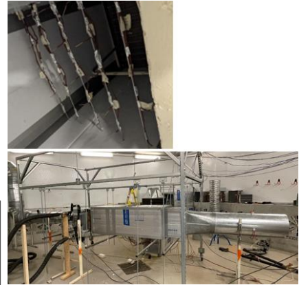
Testing apparatus diagram (left), thermocouple grid (top right), testing apparatus photo (bottom right)
