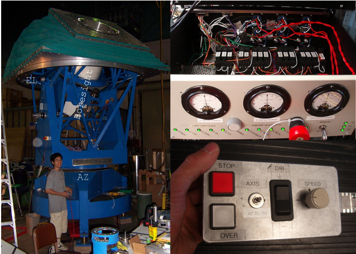
Figure 3.11: 3-axis telescope mount, interlock system, and manual controller.
