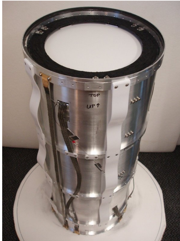
Figure 2.6: Optics tube housing two lenses at 4 K. Flexible braided copper straps were attached from the lenses to the 4 K base of the telescope enclosure for heat sinking, and the LHe vapor-cooled Teflon filter minimized the incident radiation. The edge of the top lens was measured to equilibrate at <8 K so negligible emission was expected from the lenses. Circular apertures located at the lenses and in two intermediate locations within the telescope were blackened with epoxy loaded with carbon black or iron filings to minimize stray light.
