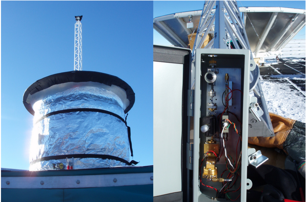
Figure 4.13: Sidelobe measurement using a modulated broadband noise source on a mast.
