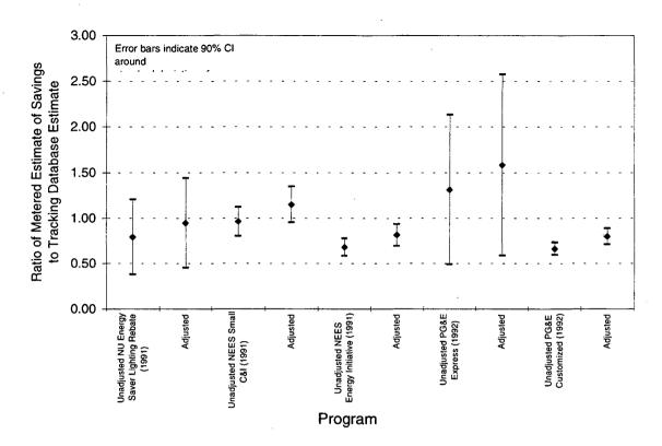
Figure 4-7. Comparison of adjusted and unadjusted metering results
