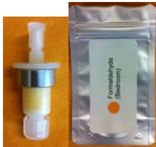
Formaldehyde sampler inside airtight bags
