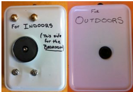
Containers for mounting air samplers in your home (Note: Lid of indoor container is for bedroom and base is for kitchen)
