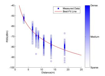
Fig. 4. An example of calibration result for a receiver.
