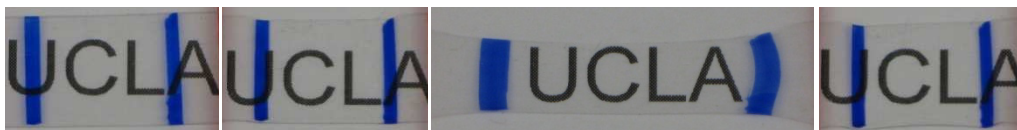
Figure 3-6. (a) A PTBA-IPN-50 membrane freshly made (distance between the blue markers are 25 mm) , (b) heated at 70°C, (c) stretched by 100% in the horizontal direction and then cooled to room temperature, and (d) reheated for 10s at 70°C.
