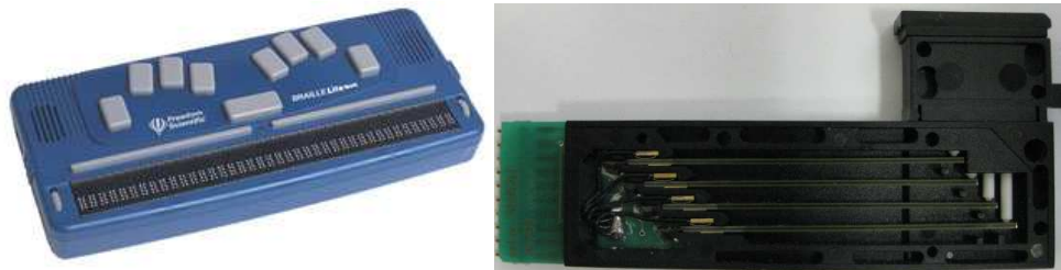
Figure 4-1. Braille Lite M40, a refreshable Braille display capable of displaying one line of text ( Left ) and the transducers (8 piezoelectric bimorphs) under a Braille cell ( Right ).
