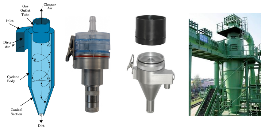
Figure 2.16: Various cyclone separator and its flow path
