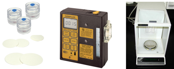
Figure 2.17: PTFE filter, sampling pump, and micro balance
