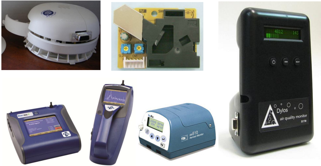
Figure 2.22: Examples of scattering based instruments: A UCB Particle Monitor [133]; B Shinyei PPD42NS dust sensor; C DustTrak II Aerosol Monitor; D SidePak Personal Aerosol Monitor; E Dylos Particle Counter
