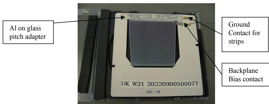
Fig. 19: A W21 Hamamatsu sensor glued to a ceramic support frame for irradiation. The sensor Al strips are wire-bonded to Al lines on a glass pitch adapter and grounded. The backplane is contacted and biased to 100 V during the irradiation.
