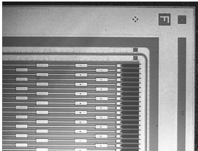
Fig. 7: Photograph of a corner of an SCT barrel silicon microstrip sensor supplied by Hamamatsu Photonics, showing the guard structure, a selection of fiducial alignment marks, the bias ring, polysilicon bias resistors, and the metallization above implant strips, including wire-bonding pads.
