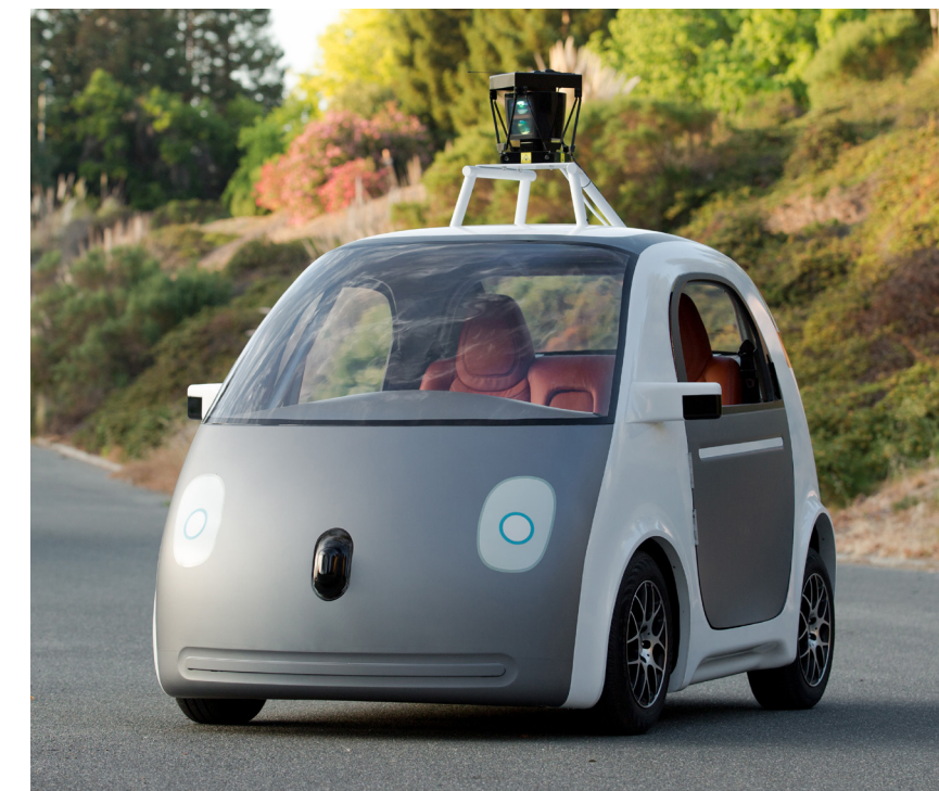
Google's most recent prototype automated vehicle concept does not include traditional driver's seat or controls - photo courtesy of Google
