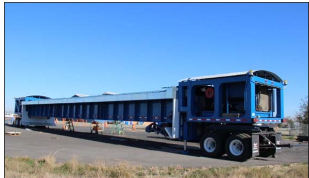
Figure 1.4: Heavy Vehicle Simulator with extended beam.
