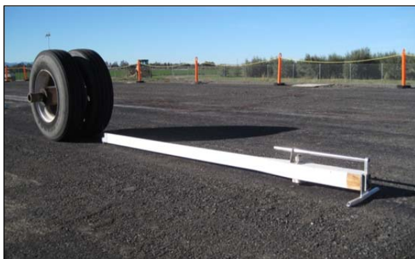
Figure 6.9: Road surface deflectometer.
