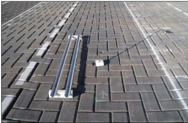
Figure 6.8: Permanent deformation measurements.
