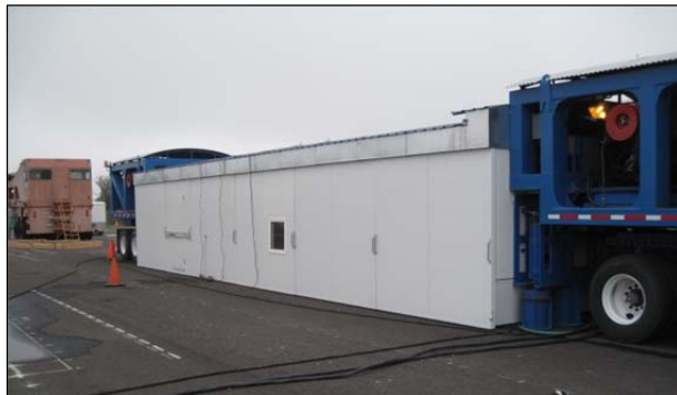
Figure 1.3: HVS with environmental chamber.
