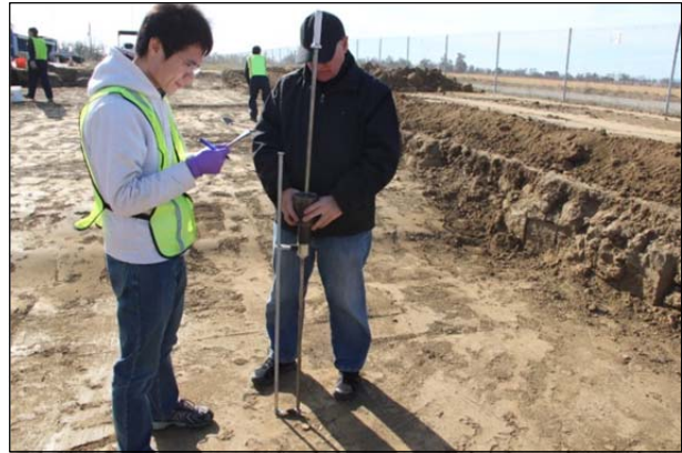
Figure 5.6: Dynamic cone penetrometer measurements.
