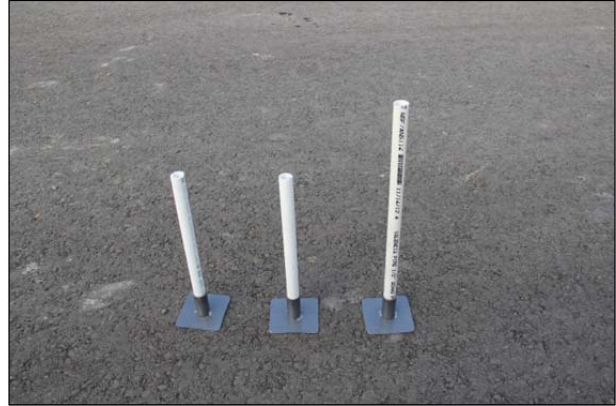
Figure 6.7: Permanent deformation gauge.
