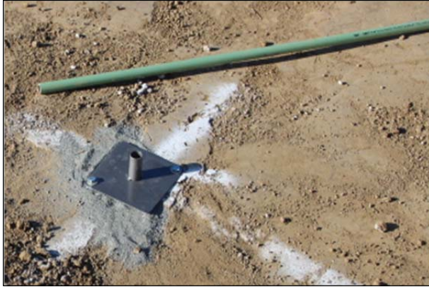
Figure 6.7: Permanent deformation gauge.
