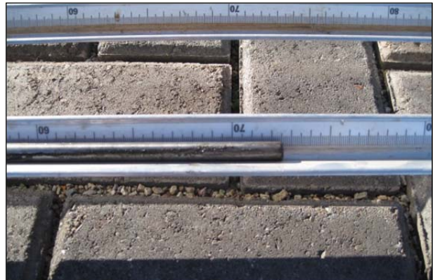
Figure 6.8: Permanent deformation measurements.
