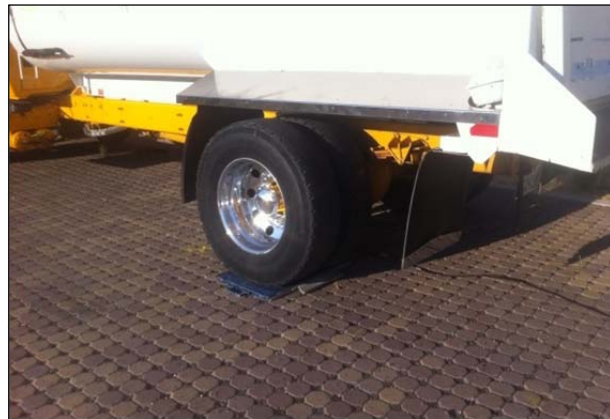
Figure 2.5: Measuring the wheel load.
