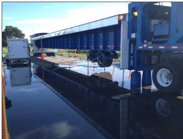
Figure 6.14: Flooded section during preparation for wet testing.
