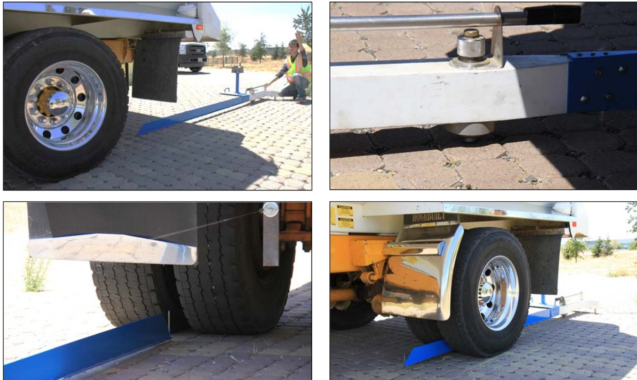
Figure 2.1: Road surface deflectometer.
