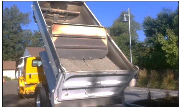
Figure 2.3: Re-distribution of aggregate to change load.
