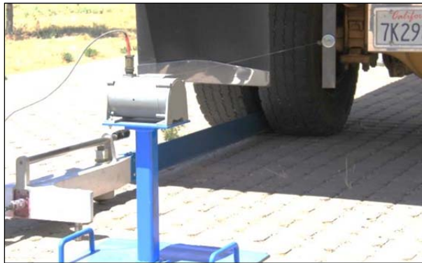
Figure 2.6: Encoder for measuring wheel location.
