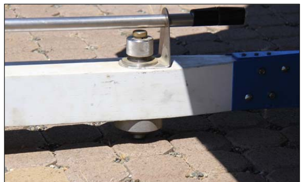
Figure 6.9: Road surface deflectometer.
