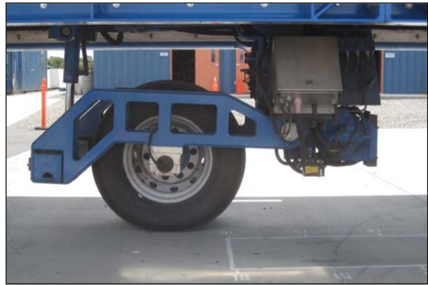
Figure 1.2: HVS test carriage.
