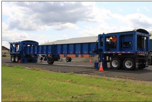
Figure 1.1: Heavy Vehicle Simulator (HVS).
