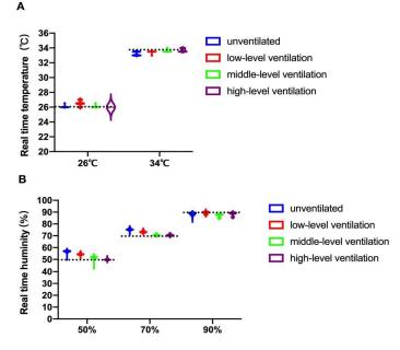
**Figure 3.** Environmental monitoring of every set of conditions. (**A**) Real-time temperature in each test cabinet with the pre-set chamber temperature of 26 °C or 34 °C; (**B**) Real-time humidity in each test cabinet with the pre-set chamber humidity of 50%, 70%, or 90% RH.
