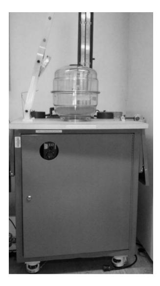
Figure 6.6: The test dome in the adaptor mode (Left) and whole glove (Right) testing modes
