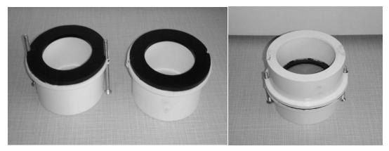
Two DANCO flush valve gaskets were cut and super-glued to the bottom of two reducer bushings to hold samples in place and to minimize water leakage.
