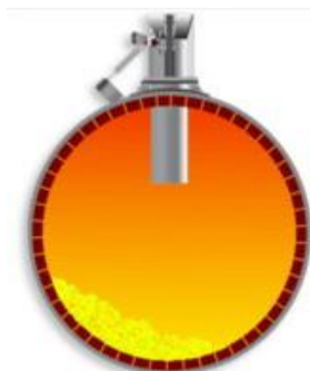
Figure 33. Cadence's mid-kiln fuel injector technology (Cadence 2012a).
