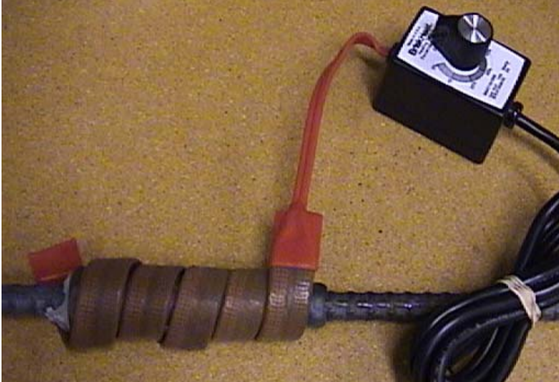
Figure 14: Photograph of epoxy-bonded rebar-coupler elevated-temperature test setup.
