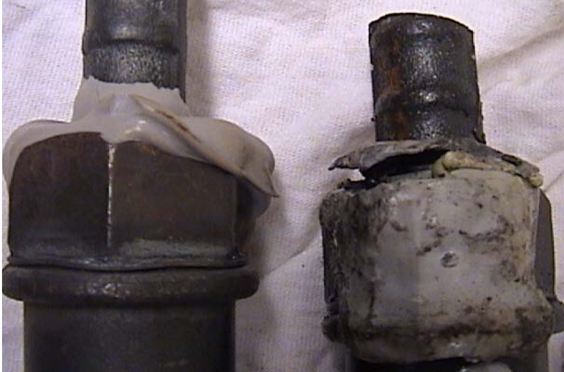
Figure 54: Photograph comparing permanent creep displacements, System C on the left, System F on the right.
