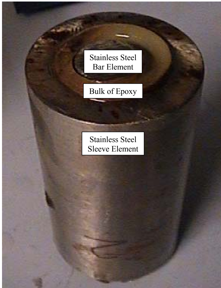
Figure 17: Photograph of moisture sleeve test specimen. Notice the stainless steel material, but with identical geometry to a typical epoxy-bonded rebar-coupler.
