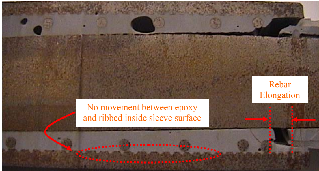
Figure 49: Photograph of a modified epoxy-bonded rebar-coupler, assembled with System C, which has been tested to failure. Elongation of the rebar is visible near the entrance of the coupler.
