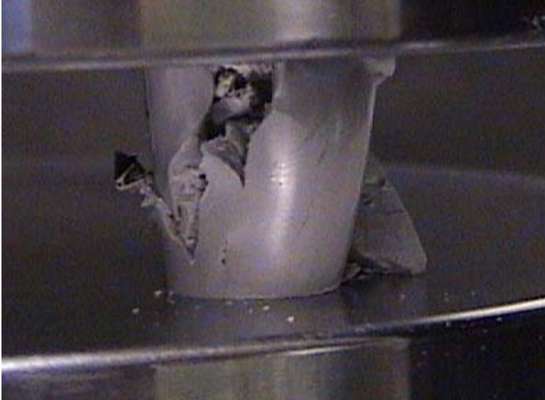
Figure 36: Photograph of cracking and crushing failure behavior of compressive test specimen.
