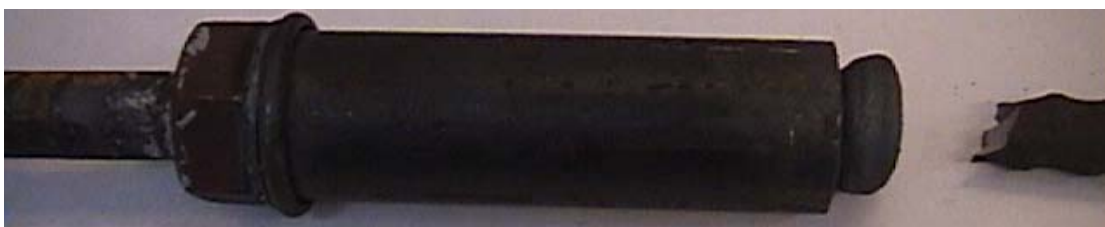
Figure 43: Photograph of an epoxy-bonded rebar-coupler, assembled with System C, which has been fatigue tested to failure. The fatigue-fracture occurred at the location of the factory rebar-to-sleeve weld at the closed end of the coupler, not adjacent to the epoxy-system.
