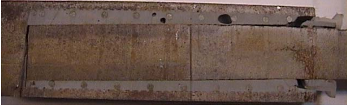
Figure 47: Photograph of a modified epoxy-bonded rebar-coupler, assembled with System C, which has been tested to failure. Some displacement at the entrance of the coupler is evinced by the movement of the plastic alignment cap. However, the movement of the embedded rebar at the back of the coupler is orders of magnitude less than that shown by the thin-walled coupler.
