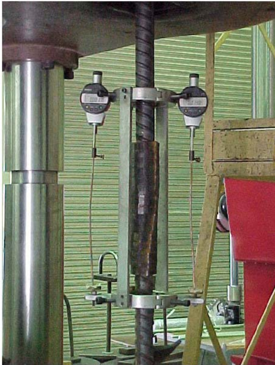
Figure 1. Example of dial indicators used for measuring slip.
