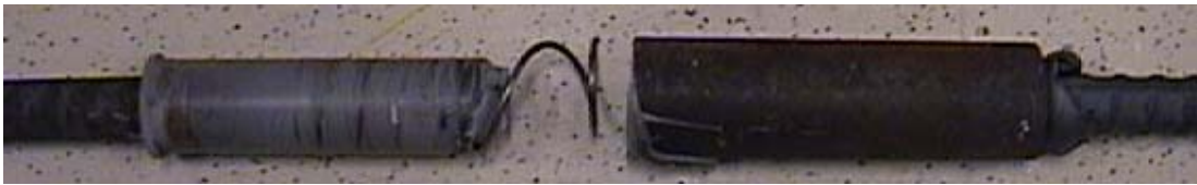
Figure 46: Photograph of a modified epoxy-bonded rebar-coupler, assembled with System C, which has been tested to failure. The lack of a choked-mouth on this coupler allowed the bulk of epoxy and embedded rebar to pull out of the coupler intact.
