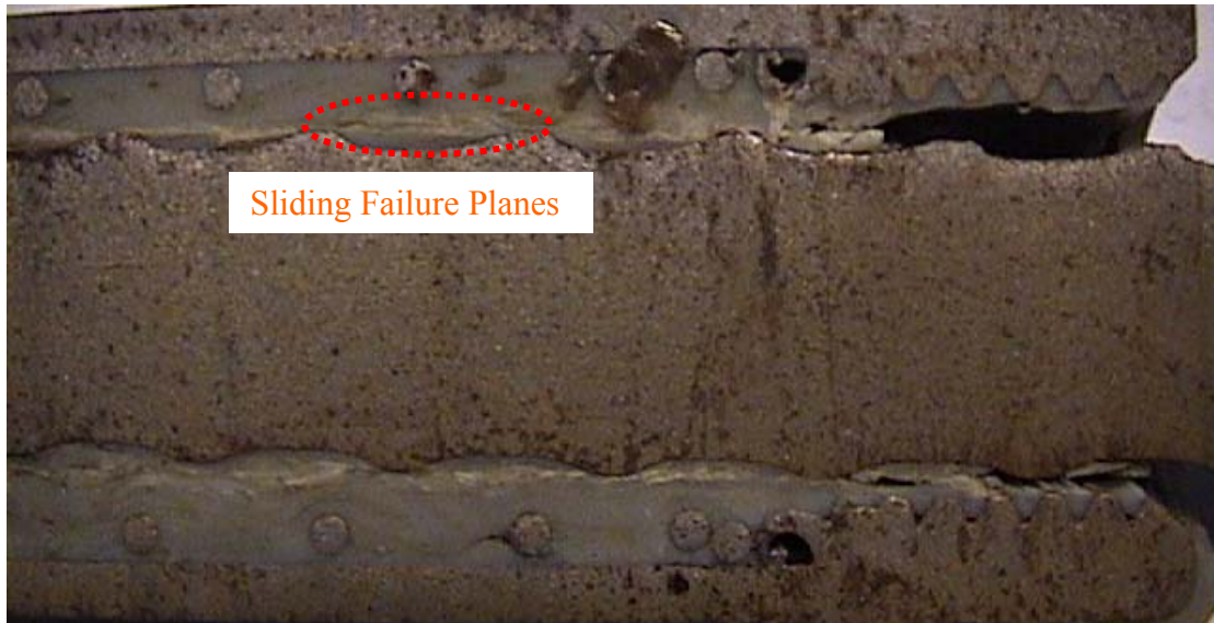
Figure 52: Photograph showing an epoxy-bonded rebar coupler, assembled with a non-optimal epoxy system, tested to failure.
