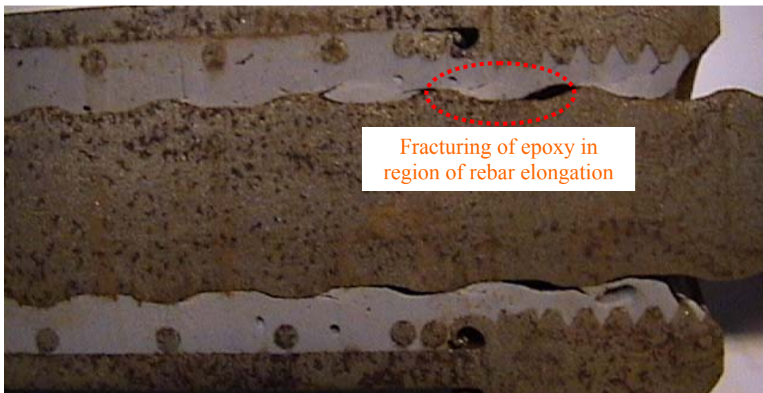
Figure 51: Photograph showing a standard epoxy-bonded rebar coupler, assembled with System C, tested to failure.
