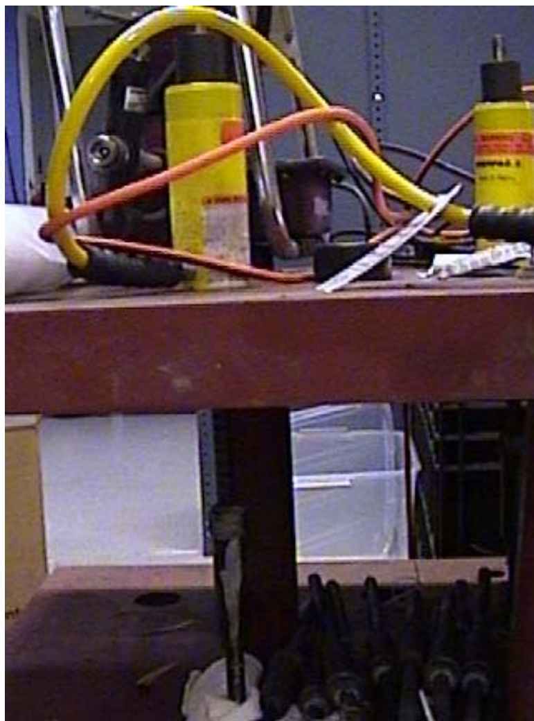
Figure 19: Photograph of rebar-coupler creep test setup.
