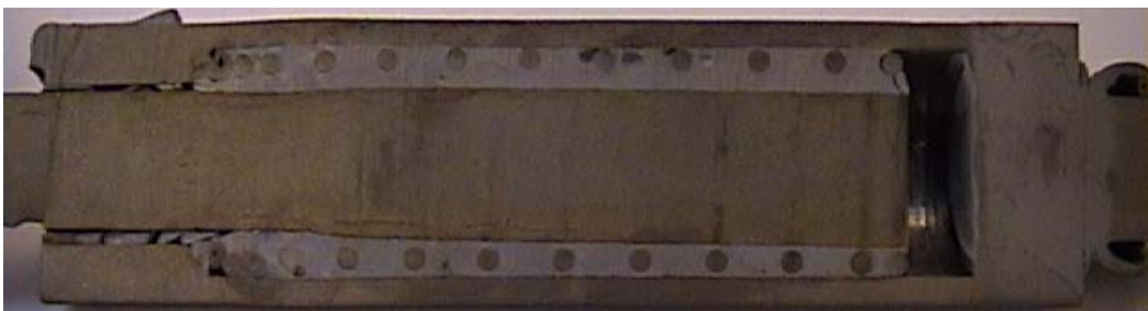
Figure 45: Photograph of a modified epoxy-bonded rebar-coupler, assembled with System C, which has been tested to failure. The thinner walls of this coupler yielded outward and created a permanent, visible bulge. Also, the bulk of epoxy, and embedded rebar, moved visibly towards the mouth of the coupler.
