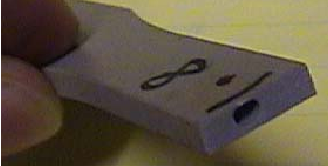
Figure 32: Photograph of fracture surface, including air void, of tensile test specimen. Voids can contribute to variability of tensile test results.
