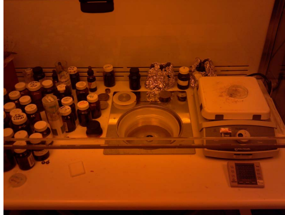
Figure 4.1. Headway PWM32 spinner. Resist is spun onto the substrate at speeds of 3000 - 5000 RPM using the Headway PWM32 spinner. The spinner resides in an overpressured hood which prevents particle contamination. The resist is baked onto the sample using the temperature-regulated hot plate next to the spinner. The yellow lighting in the room prevents unwanted exposure of photoresist due to ultraviolet light.
