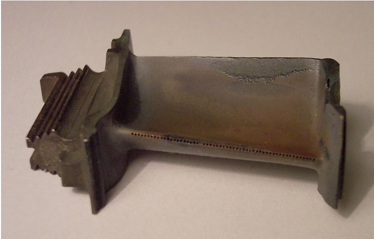
Figure 2.2: Gas turbine blade constructed of single-crystalline Ni-based superalloy [45].
