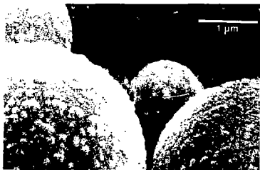
Figure 4. High magnification scanning electron micrograph of surface of fly ash particles. Marker shows 1 \mu m. XBB 780-13879 (Magnification = 17,000 \times )
