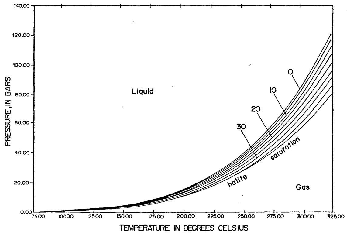
Figure 5.4 Saturation curve for  $\text{H}_2\text{O}-\text{NaCl}$  system (after Haas, 1976).
