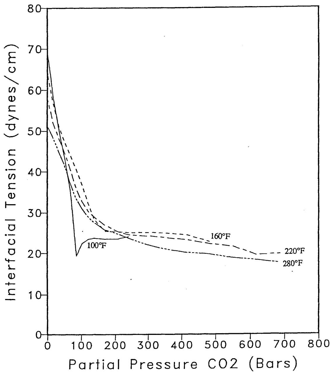
Figure 5.3 Effect of CO<sub>2</sub> on the surface tension of H<sub>2</sub>O at different temperatures.
