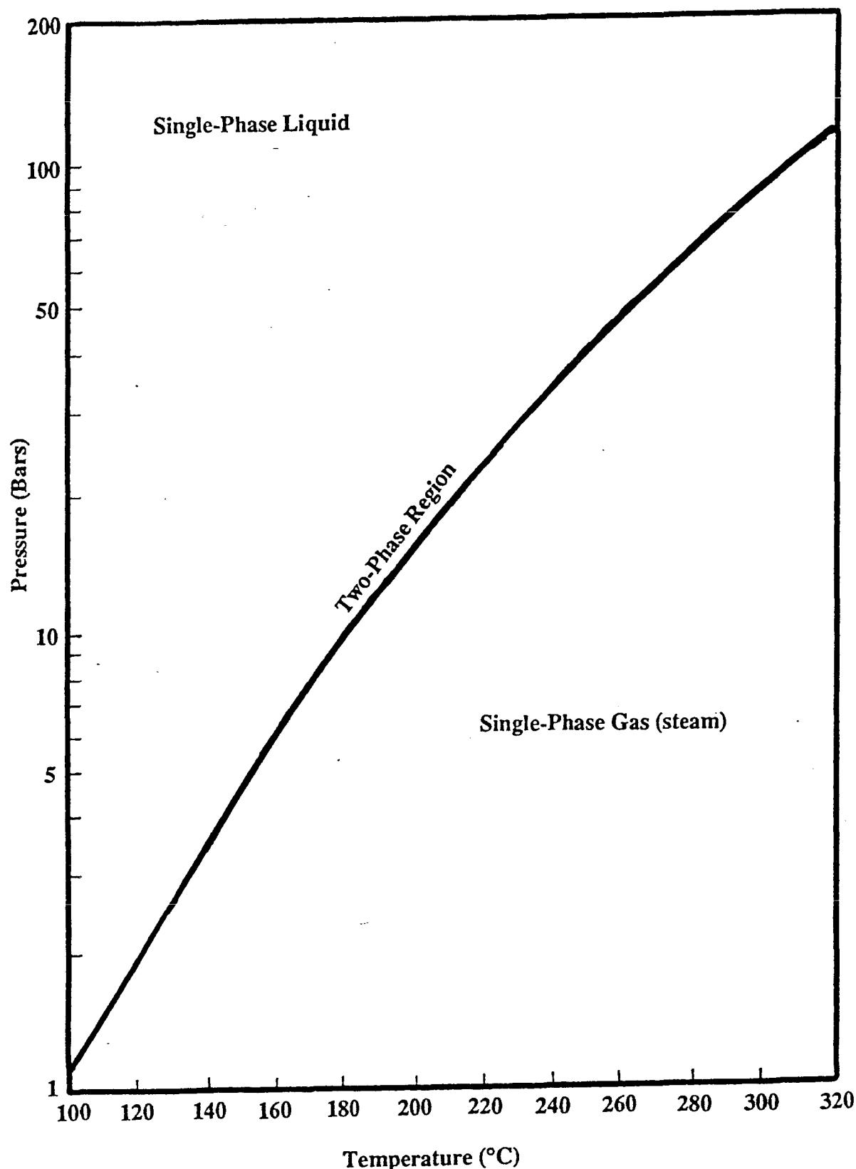
Figure 5.1 Saturation curve for  $\text{H}_2\text{O}$  (after Pritchett et al., 1981).
