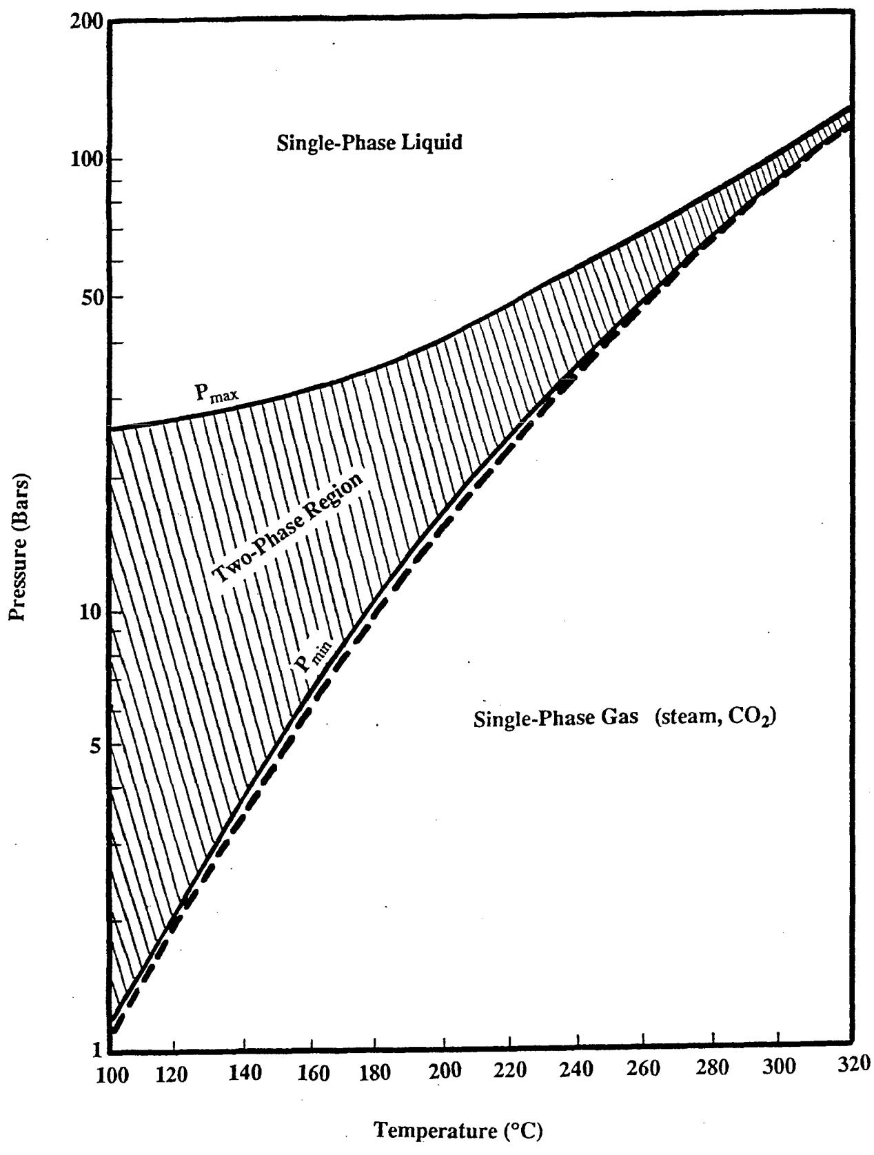
Figure 5.2 Saturation curve for  $\text{H}_2\text{O}-\text{CO}_2$  system with 1%  $\text{CO}_2$  (after Pritchett et al., 1981).
