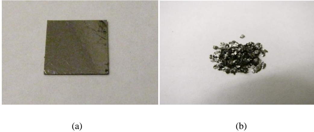
Figure IV-5 Optical microscope image of HOPG (a) and Kish Graphite (b).
