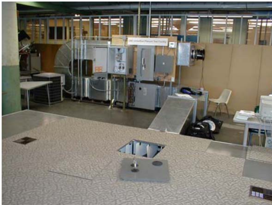
Figure 2-21 Experimental Test Equipment for Plenum Model Validation
