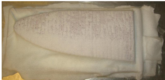
Figure 5.20: Vacuum bag removed, before removing breather cloth and peel ply.
