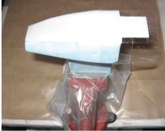
Figure 5.3: Foam mold prepared for wet layup process.
