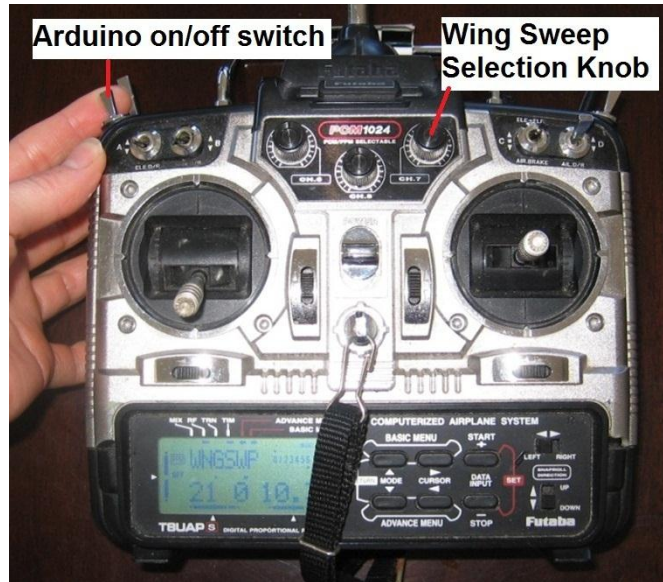
Figure 6.4: The RC transmitter set up for manual sweep control.
