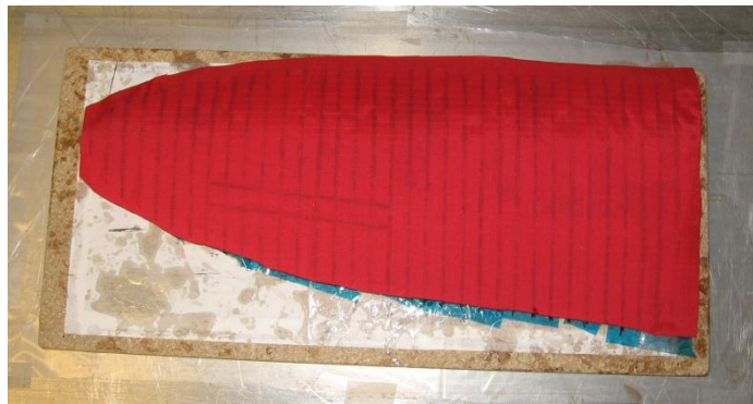
Figure 5.16: Rip-stop nylon applied on top of carbon strips and fiberglass layers.
