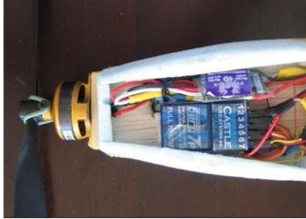
Figure 5.39: RC electronics in nose of aircraft
