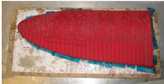
Figure 5.22: Part after vacuum bagging cloth removed.
