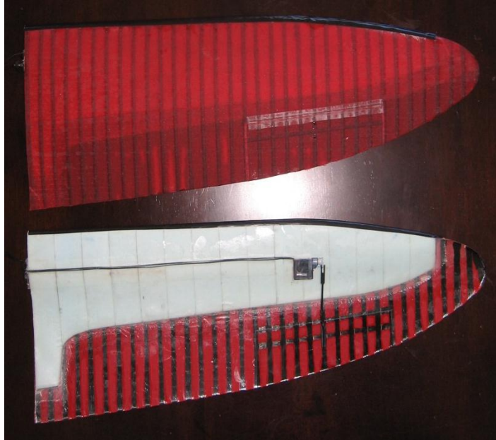
Figure 5.28: Completed wings with ailerons and attachment points.
