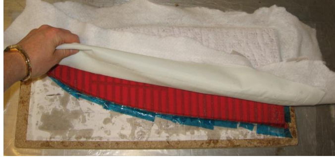
Figure 5.21: Removing breather cloth and peel ply.
