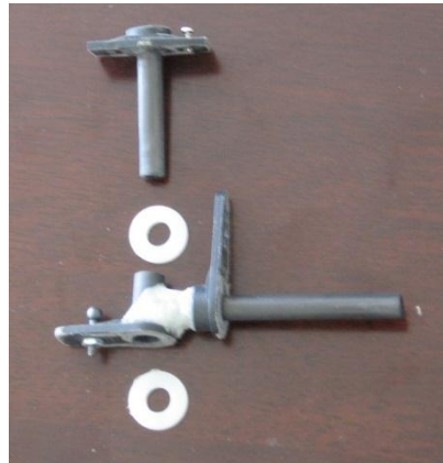
Figure 5.32: Carbon shoulder joint components
