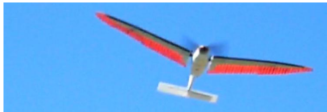
Figure 7.1: Aircraft flying with wings in neutral sweep position.
