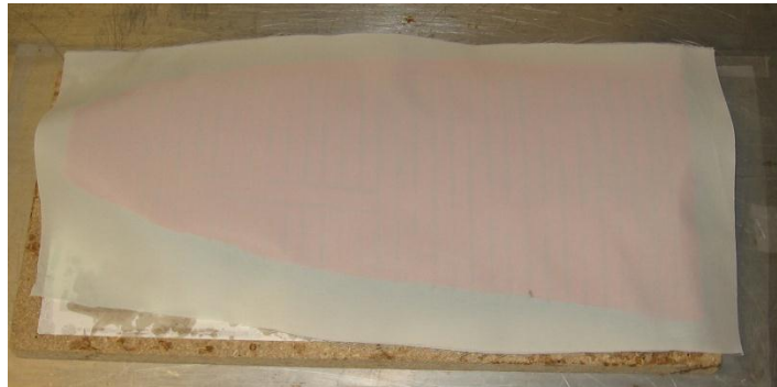
Figure 5.17: Peel ply draped over the part.
