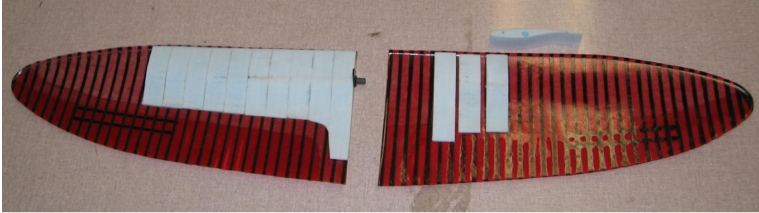
Figure 5.26: Building the bottom foam structure.
