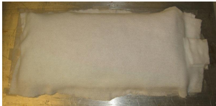
Figure 5.18: Breather cloth draped over the mold.
