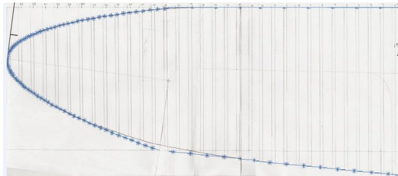
Figure 3.4: Final wing planform after tiling parabolic tip section.
