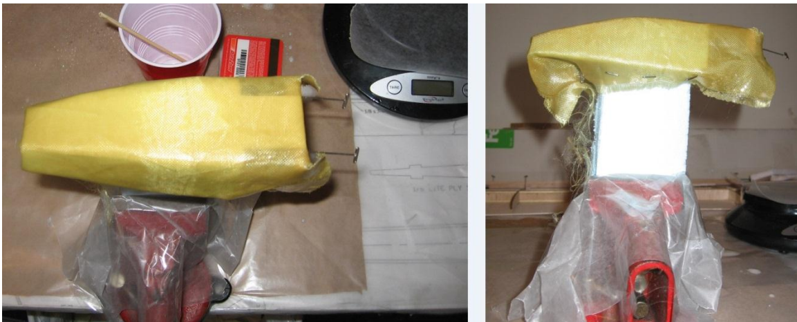
Figure 5.4: Kevlar pinned to foam mold.
