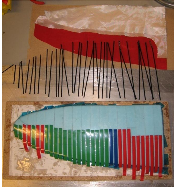
Figure 5.12: Materials cut and prepared for wet layup.
