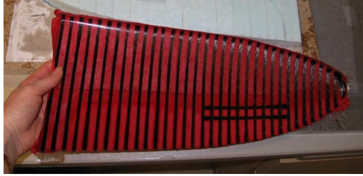
Figure 5.24: Part after removing release film.
