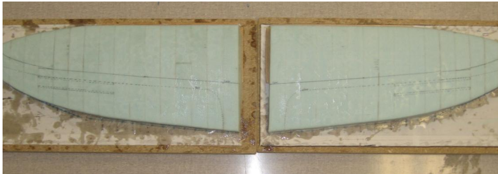
Figure 5.10: Completed molds with fiberglass applied and guidelines drawn.
