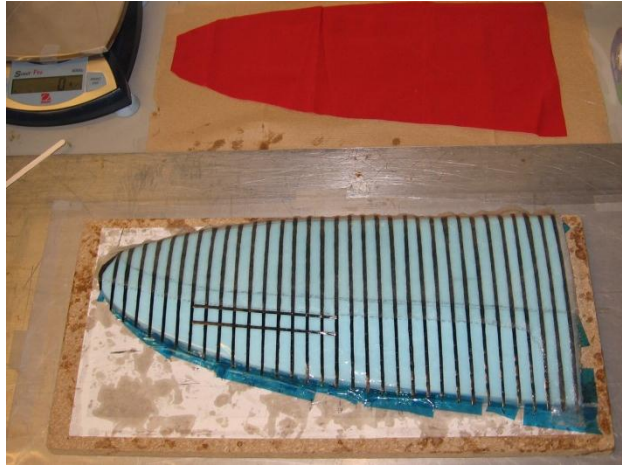
Figure 5.15: Fiberglass applied to mold (wetted glass is clear).
