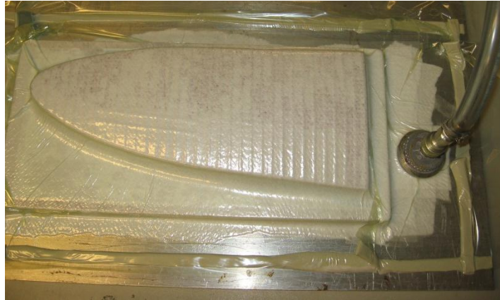
Figure 5.19: Part curing in a vacuum bag.
