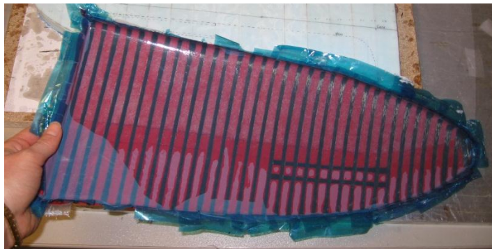
Figure 5.23: Underside of part, before removing release film.
