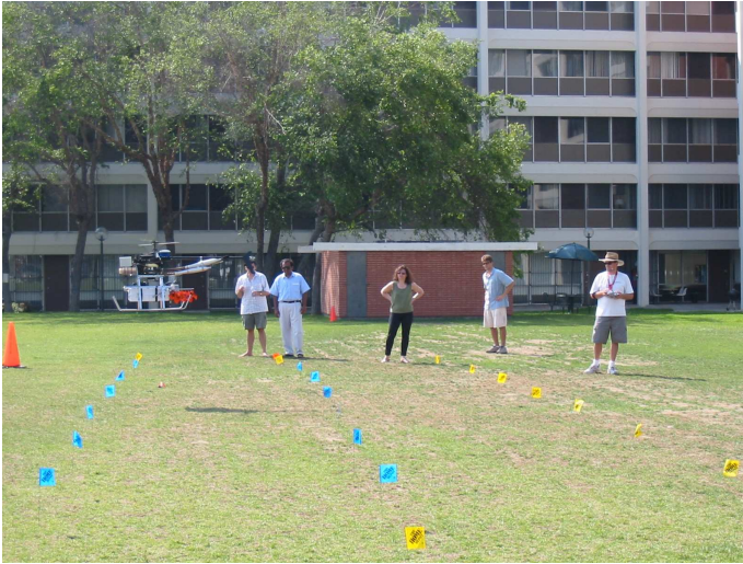
Fig. 3. Helicopter Deploying Sensors in a 7 \times 7 grid
