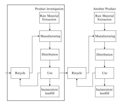
Fig. 10.3 The allocation procedure for open-loop recycling
