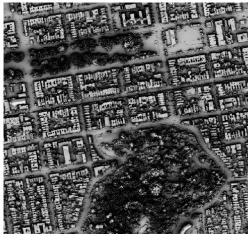
Figure 5.2 Example of DSM derived from LiDAR, San Francisco
