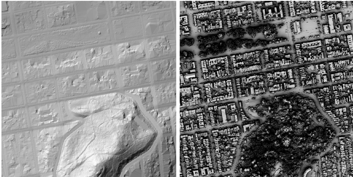
Figure 4.5 Digital Elevation Model (DEM) and DSM derived from LiDAR
