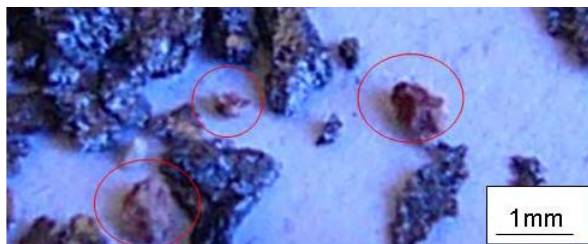
Figure 4.55 Reddish fragments observed among regular black scattered pieces after dynamic testing and comminution of C_{Pitch}/Al-Mg sample bulk damaged at high strain rate ( 5000 or 7000\text{ s}^{-1} ).
