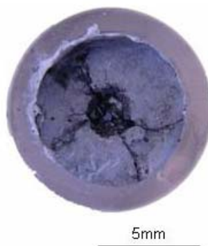
Figure 4.6 The nearly collapsed sample from the mixture of PTFE and 2- \mu\text{m} Al in polymer jacket. Note the characteristic four cracks/shear bands.
