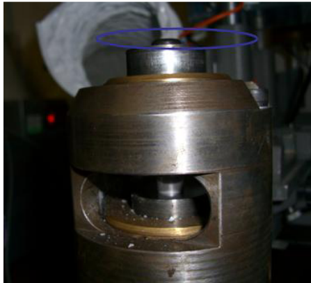
Figure 3.16 Polymer o-ring (black in the circle) was placed on the top of the upper anvil to mitigate parasitic oscillations.
