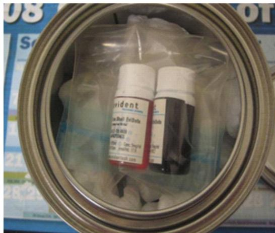
**Figure 3.2:** The near infrared PbS QDs (Right) and the visible CdSe/ZnS QDs (Left) for prototyping of LSCs provided by the Evidot vendor. They are dispersed in toluene.
