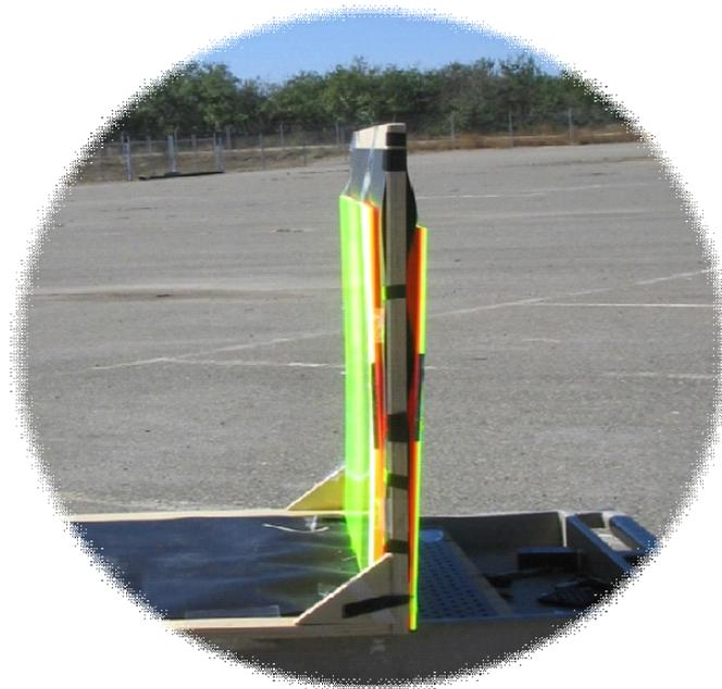
**Figure 4.35:** Experimental set up for the performance of LSCs in collecting global and diffuse light. Prototypes of LSCs are fabricated by stacking green and red LSCs together.
