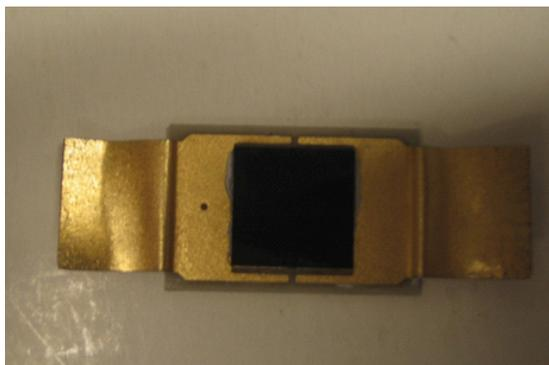
**Figure 3.6:** The solar cell as a detector for the electrical characterization of LSC concentration factors. It is produced by SunPower Company. The left and right sides are two electrodes.
