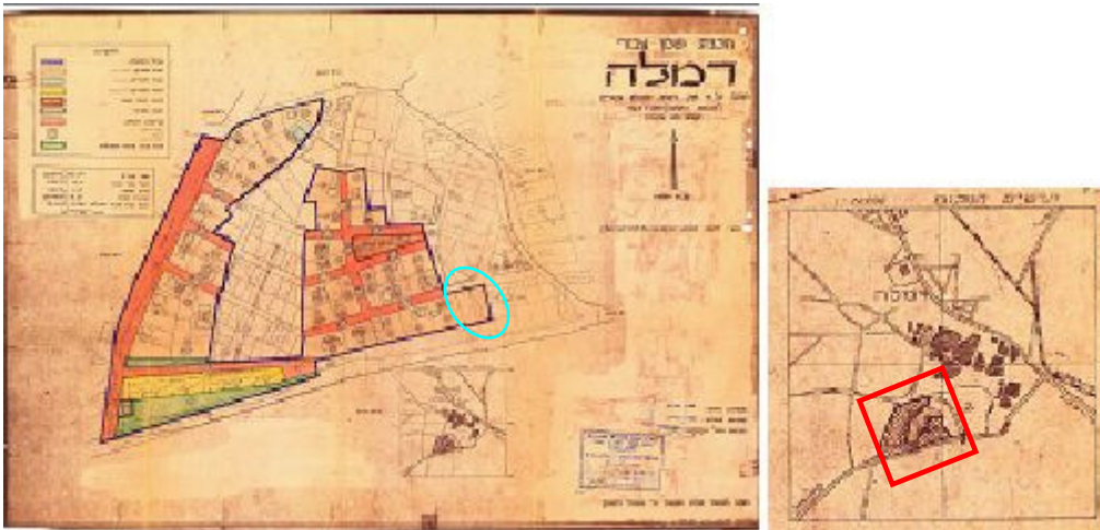
Fig. 6.32, 6.33 Ramla public housing plan, prepared by the law of public housing registration, 1964. The plan regulates the 1964 condition of original shacks (in brown, right plan) and new structures (in blue contour). Source: ILA. The Ninio shack is on parcel 41, marked in turquoise by me. It is important to note that the plan was outlined long after the neighborhood had been populated, in 1964, for the purpose of registering immigrant housing and enabling them to purchase their housing from the state and register it to their name if already purchased. 1031
