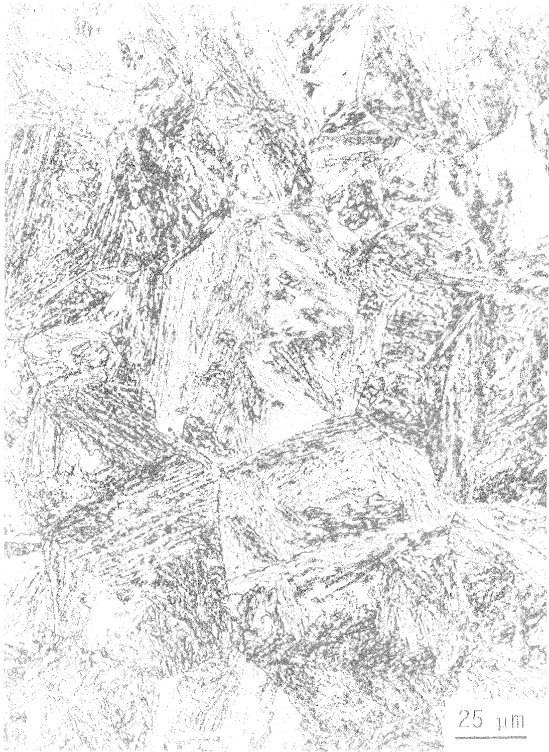
Figure 32. Micrograph showing bainitic microstructure in Cr-Mo steel modified with 0.5% Ni and an additional 0.5% Mn.
