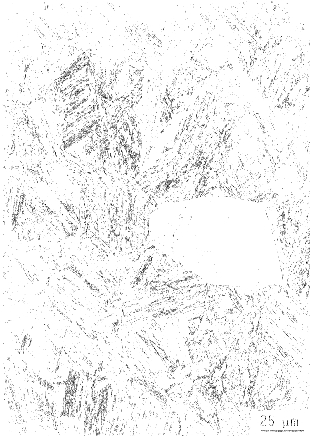
Figure 36. Optical microscope of Cr-Mo steel with additional Ni, Mn and Si. Fine areas of ferrite are present.
