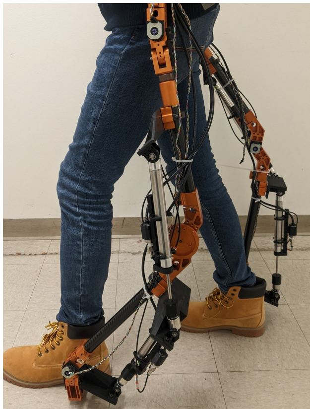
Figure 2.3: The backward-knee pneumatic exoskeleton developed in Bionics Lab, UCLA.
