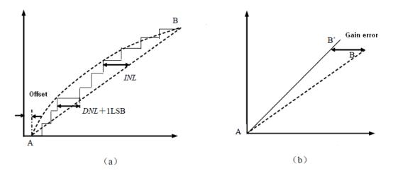
Figure 1.4 ADC Static Errors.
