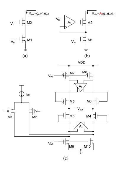
Figure 3.18(a, b) Gain Boosting Technology, (c) Folded-cascode Op-amp with Gain
