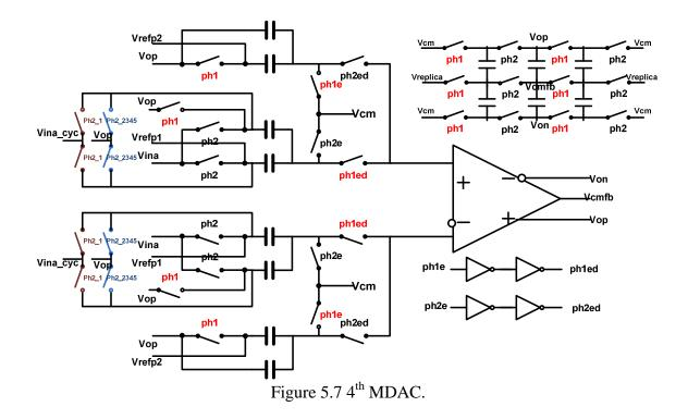
Using 1~5 counter to control the switches during cyclic processing.
