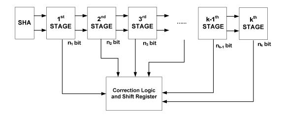
Figure 4.8 Pipeline ADC Structures.
