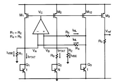
Figure 3.23 Curvature-compensated BGR.
