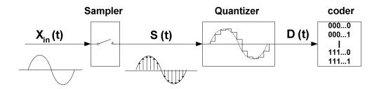
Figure 1.3 Analog-to-Digital Converter Block Diagram.
