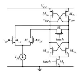
Figure 3.11 Class-AB Latched Comparator.
