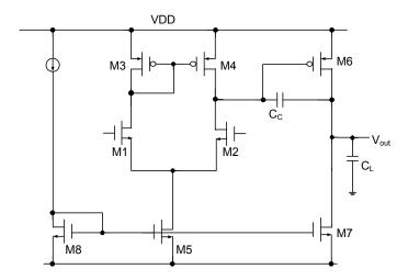
Figure 3.15 Two-stage Op-amps.
