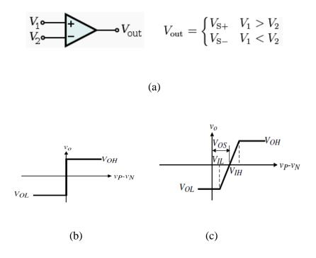
Figure 3.6 (a) Comparator Symbol (b) Ideal Transform Function
