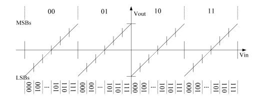
Figure 3.1 Pipeline ADC Transfer Curve.
