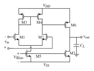
Figure 3.7 Amplifier-type Comparator.
