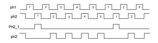
Figure 5.8 Phase Scheme of Cyclic ADC.
