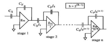
Figure 4.3 Capacitor Scaling Down.
