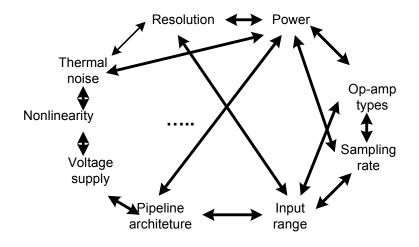
Figure 3.4 Pipeline ADC Design Matrix.
