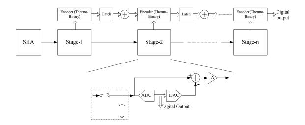
Figure 3.3 Detailed Pipeline ADC Architecture.
