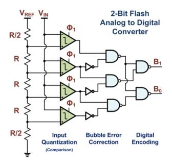
Figure 2.1 A Typical Structure of A Flash ADC.
