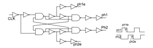
Figure 5.2 Non-overlapping Clock Generator.
