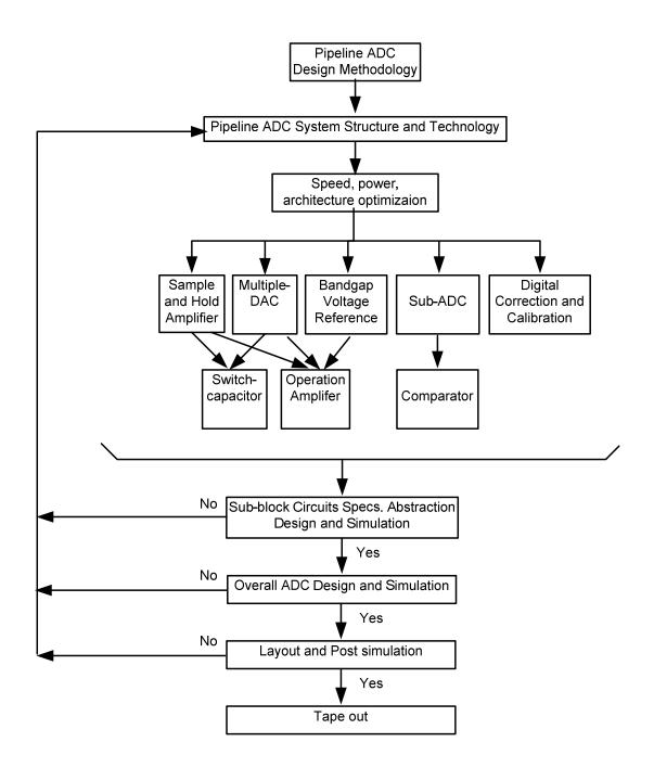
Figure 3.5 Pipeline ADC Design Flow.
