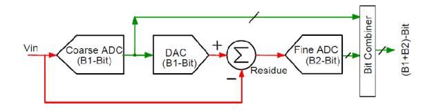
Figure 2.2 Two-Step Flash ADC.
