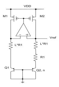
Figure 3.22 Bandgap Voltage Reference.
