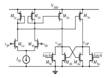
Figure 3.10 Static Latched Comparator.
