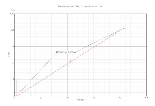
Figure 5.11 Ramp Signal to Verify Monotonicity.
