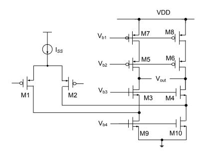
Figure 3.17 Folded-cascode Op-amps.
