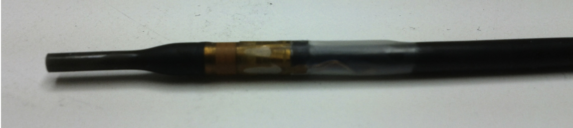
Figure 5.2: Intravascular ultrasound (IVUS) transducer used in studies in this chapter (Visions, Volcano Therapeutics, Rancho Cordova, CA). IVUS transducers are typically single- or multi- element linear arrays that mechanically rotate to create a 360^\circ image, whereas the transducer used in our studies was radially phased (gold section in figure), with 64 elements placed around the circumference of the catheter.
