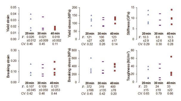
**Figure 24** Comparison of tensile properties of silk samples collected from a single white cocoon and microwaved for 20 minutes, 30 minutes, or 40 minutes. The conventionally calculated mean  $(\bar{x}) \pm$  standard deviation is given below each set of samples (in the same units as the plotted data), along with the coefficient of variation (CV).
