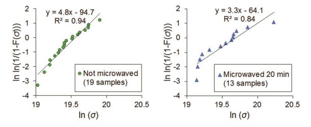
**Figure 29** Weibull plots constructed with the breaking strength of samples that had not been microwaved (left), and samples with 20 minutes of microwave exposure (right).
