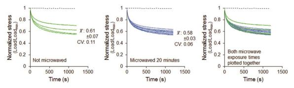
**Figure 28** Stress relaxation in silkworm cocoon silk with 0 minutes (4 samples) and 20 minutes (9 samples) of microwave exposure. Initial ramp rate was doubled relative to the tests plotted in Figure 27. The conventionally calculated mean  $(\bar{x}) \pm$  standard deviation of the normalized stress at the end of the test is given for each batch of silk, along with the coefficient of variation (CV). The horizontal broken line was obtained from carbon fiber.
