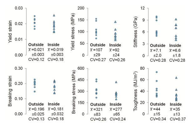
**Figure 9** Comparison of tensile properties of silk samples taken from the outside and inside surfaces of a cocoon. The mean  $(\bar{x}) \pm$  standard deviation is given below each set of samples (in the same units as the plotted data), along with the coefficient of variation (CV). The ambient testing temperatures for outside and inside samples were 21.2  $\pm$  0.4 °C and 21.1  $\pm$  0.4 °C, respectively, and the relative humidities were 45  $\pm$  3% and 46  $\pm$  4%, respectively.
