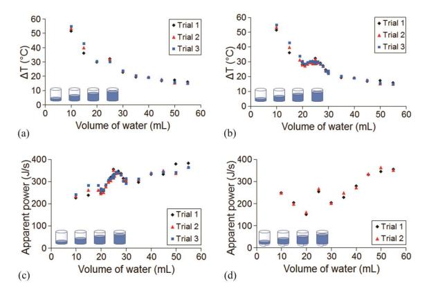
**Figure 19** (a) Temperature increase caused by microwaving fixed volumes of water in a 50 mL beaker. (b) Additional data collected in the vicinity of the anomalous peak at ca. 25 mL. (c) Corresponding estimates of the microwave oven output power, obtained with Equation 1. (d) The effect of raising the beaker by 10 mm. The microwave oven timer was set to 12 s in all cases.
