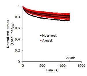
**Figure 35** Comparison of stress relaxation in samples that had not been annealed ("No anneal."), and samples that had been annealed ("Anneal."). At the time of testing, the ambient temperature was 23.6 °C  $\pm$  0.2 °C ("No anneal."), and 23.5  $\pm$  0.2 °C ("Anneal."). The ambient humidity was 47%  $\pm$  1% and 46%  $\pm$  1% respectively.
