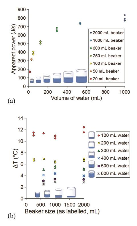
**Figure 18** (a) Estimated microwave oven output power (using Equation 1) as a function of water volume and beaker size (fixed aspect ratio). (b) Temperature increase caused by microwaving fixed volumes of water in different sizes of beaker (different aspect ratios). The microwave oven timer was set to 12 s in all cases.
