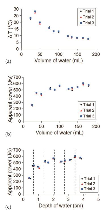
**Figure 21** (a) Temperature increase caused by microwaving fixed volumes of water in a 300 mL Erlenmeyer flask. (b) Corresponding estimates of the microwave oven output power, obtained with Equation 1. (c) Microwave oven output power plotted as a function of the depth of water used in the Erlenmeyer flask; depths that may accommodate standing microwaves (Equation 11) are indicated with dashed lines. In all cases the microwave oven timer was set to 12 s.
