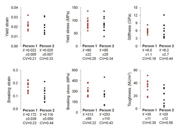
**Figure 13** Comparison of tensile properties of silk samples collected by two different people. The mean ( $\bar{x}$ ) ± standard deviation is given below each set of samples (in the same units as the plotted data), along with the coefficient of variation (CV). The ambient temperature and humidity during testing were approximately 23°C and 54% respectively.
