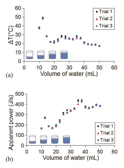
**Figure 20** (a) Temperature increase caused by microwaving fixed volumes of water in a 100 mL beaker. (b) Corresponding estimates of the microwave oven output power, obtained with Equation 1. The microwave oven timer was set to 12 s in all cases.
