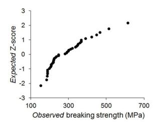
**Figure 8** Normal probability plot constructed with breaking strength data collected from silkworm silk that has been microwave irradiated. Nonlinearity indicates the data does not follow a normal distribution.
