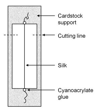
**Figure 3** Silk sample glued to a cardstock support. The gauge length of the sample is defined by the distance between points of attachment to the cardstock support—i.e. the length of silk spanning the hole in the cardstock support, between the dots of cyanoacrylate glue.
