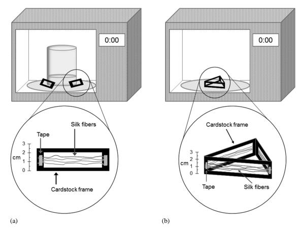
**Figure 2** Schematic representation of silk fibers ready for exposure to microwave radiation: (a) with a water load included in the microwave oven as a "sink" for excess microwave radiation, and (b) without such a water load.
