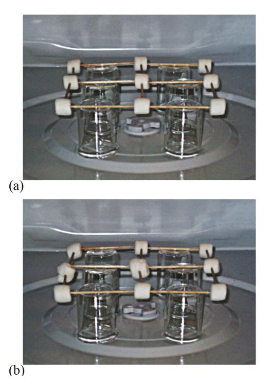
**Figure 22** (a) Marshmallows joined by toothpicks and resting on inverted 25 mL beakers in the microwave oven (no turntable present). (b) After microwaving for a few seconds, some (not all) of the marshmallows have begun to melt.
