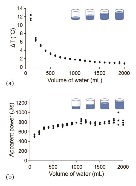
**Figure 17** (a) Temperature increase caused by microwaving different volumes of water in a 2 L beaker for a set time of 12 s. A minimum of four trials were performed (and plotted here) for each volume of water tested. (b) Corresponding estimates of the microwave oven output power, obtained with Equation 1.
