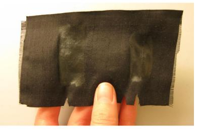
**Figure 31** A piece of silk fabric, with one thermochromic liquid crystal paint on the left (active in the 95-104°F range), and another on the right (active in the 104-113°F range).
