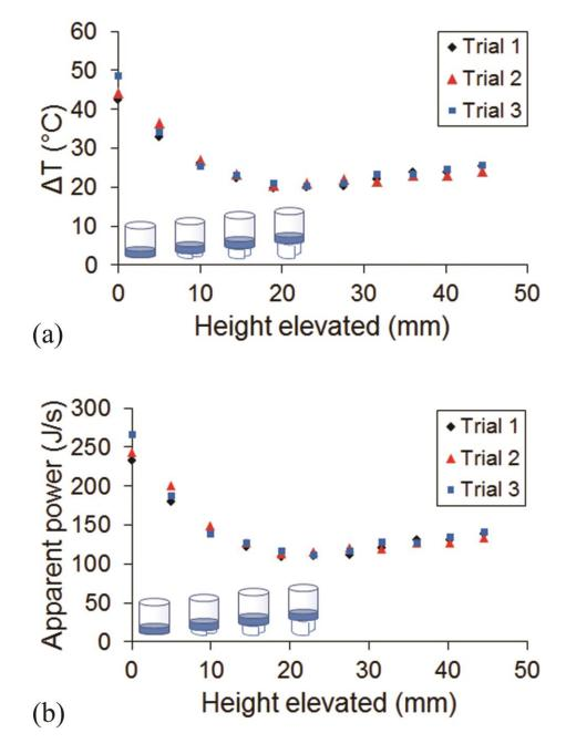
**Figure 23** (a) Temperature increase caused by microwaving 12.5 mL of water in a 50 mL beaker, plotted as a function of the height of the beaker above the turntable. (b) Corresponding estimates of the microwave oven output power, obtained with Equation 1. The microwave oven timer was set to 12 s in all cases.
