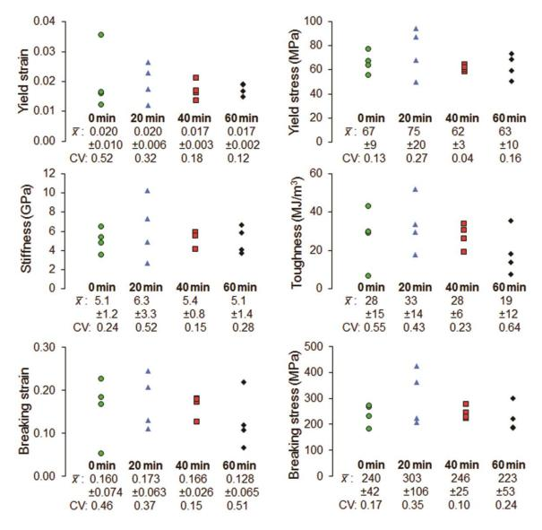
**Figure 26** Comparison of tensile properties of silk samples collected from a single yellow cocoon and microwaved for 0 minutes, 20 minutes, 40 minutes, and 60 minutes (4 samples in each case). No water load was included in the microwave oven. The conventionally calculated mean  $(\bar{x}) \pm$  standard deviation is given below each set of samples (in the same units as the plotted data), along with the coefficient of variation (CV).
