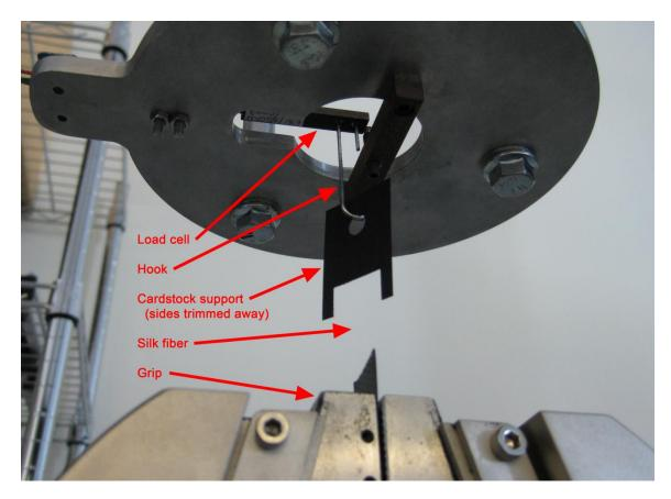
Figure 6 View of the connection between the sample (mounted on a cardstock support) and the cantilever load cell.
