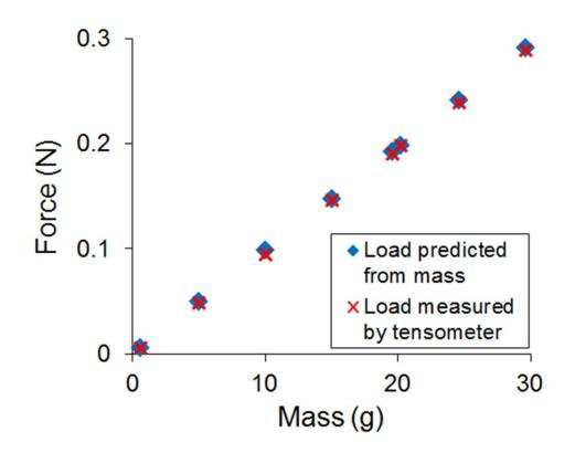
Figure 7 A comparison of loads as measured by the calibrated tensometer when weights are hung from it, and as predicted by Newton's second law based on the known masses of the weights.
