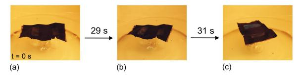
Figure 33 Thermochromic liquid crystal paints on silk fabric change color as microwave exposure time progresses.
