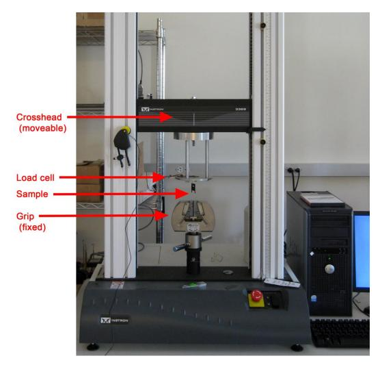
Figure 5 Instron tensile tester equipped with a 0.5 N cantilever beam load cell.
