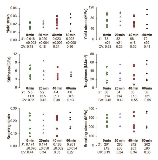
**Figure 25** Comparison of tensile properties of silk samples collected from a single yellow cocoon and microwaved for 0 minutes (6 samples), 20 minutes (5 samples), 40 minutes (6 samples), and 60 minutes (5 samples). The conventionally calculated mean ( $\bar{x}$ ) ± standard deviation is given below each set of samples (in the same units as the plotted data), along with the coefficient of variation (CV).
