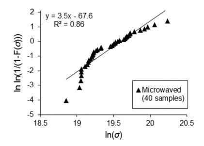
**Figure 30** Weibull plot constructed with the breaking strengths of samples that had been microwaved for times ranging from 20 to 60 minutes.
