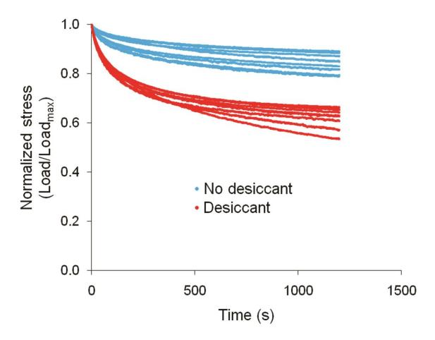
**Figure 11** Comparison of stress relaxation in samples that had been stored without desiccant and with desiccant. Ambient testing temperatures for samples that had been stored without and with desiccant were  $21.3 \pm 0.4^{\circ}$ C in both cases, and the relative humidities were  $34 \pm 6\%$  in both cases.
