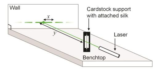
Figure 4 Schematic representation of Fraunhofer diffraction used to measure the diameter d of silk samples; x is the distance measured on the wall from the direct beam of the laser to the first dark node. The distance y between the sample and the wall was fixed at 1 m. The laser beam is normal to the plane of the wall, so that x and y are perpendicular to each other.
