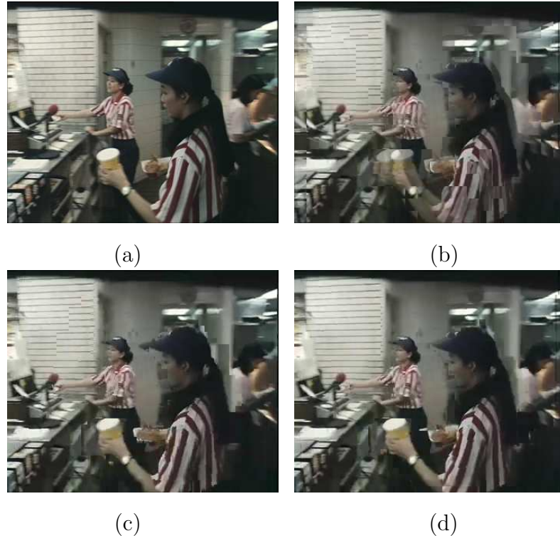
Figure 5.7: The interpolated results of frame 192 of FAST FOOD using (a) original frame, (b) direct MCFI (PSNR: 23.70dB, SSIM: 0.8035), (c) The method in [4] (PSNR: 27.12dB, SSIM: 0.8925), and (d) the proposed method (PSNR: 27.53dB, SSIM: 0.9257).
