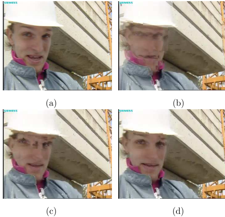
Figure 5.9: The interpolated results of frame 174 of FOREMAN using (a) original frame, (b) direct MCFI (PSNR: 27.33dB, SSIM:0.8598), (c) The method in [4] (PSNR: 29.32dB, SSIM: 0.9212, and (d) the proposed method (PSNR: 31.00dB, SSIM: 0.9449).
