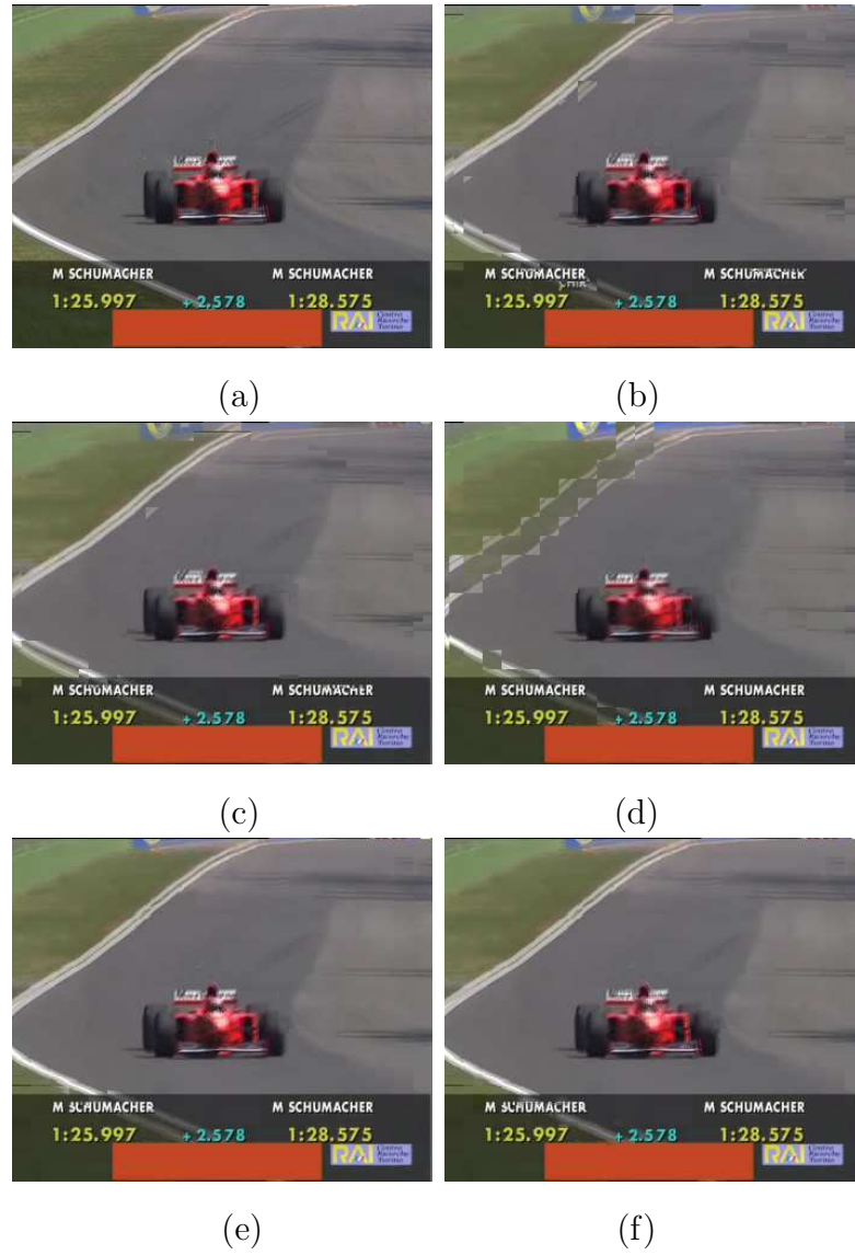
Figure 4.7: The interpolated results of frame 52 of FORMULA 1 using (a) original frame, (b) direct interpolation (PSNR: 30.53dB, SSIM: 0.9430), (c) VMF (PSNR: 30.50dB, SSIM: 0.9446), (d) bidirectional BMA (PSNR: 26.83dB, SSIM: 0.8278), (e) the proposed correlation-based MV processing with the bidirectional MCFI scheme (PSNR: 33.52dB, SSIM: 0.9681), and (f) the proposed correlation-based MV processing method with the proposed MCFI scheme (PSNR: 32.66dB, SSIM: 0.9632).
