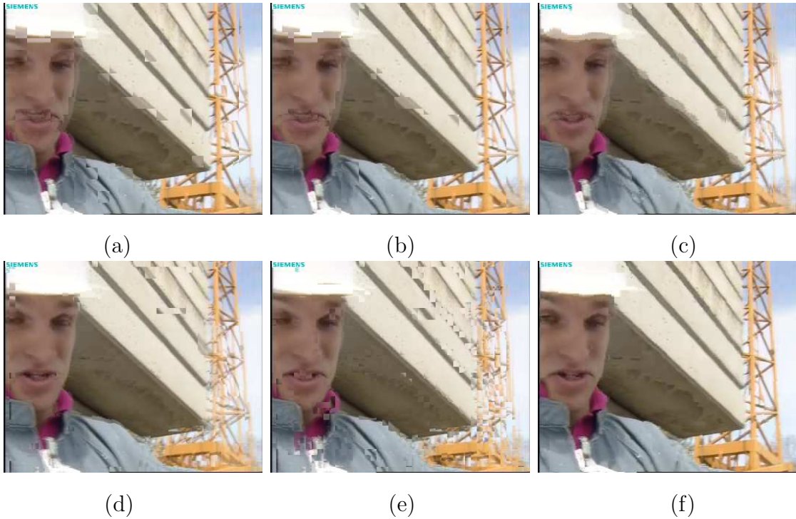
Figure 1.6: The interpolation frames of FOREMAN frame 182. (a) Direct MCFI. (b) VMF. (c) MV smoothing [1]. (d) Multisize BMA [2]. (e) Adaptive VMF [3]. (f) The proposed method [4]. Here, adaptive VMF is implemented at decoder with a prior full-search motion re-estimation based on the block size of 8 \times 8 .
