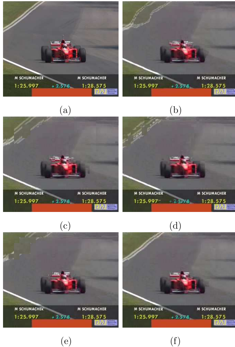
Figure 3.14: The interpolated results of frame 56 of FORMULA 1 using (a) original frame, (b) MV smoothing (PSNR: 29.46dB, SSIM: 0.9013), (c) VMF (PSNR: 29.80dB, SSIM: 0.9067), (d) multi-size block matching algorithm (PSNR: 29.85dB, SSIM: 0.9149), (e) proposed MV selection (PSNR: 30.23dB, SSIM: 0.9225), and (f) the proposed multi-stage MV processing method (PSNR: 31.56dB, SSIM: 0.9567).
