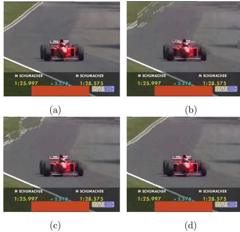
Figure 3.18: The interpolated results of frame 56 of FORMULA 1 using (a) the original frame 56, (b) direct MCFI (PSNR: 29.68dB), (c) the proposed method without color consideration (PSNR: 29.58dB), and (d) the proposed method with color consideration (PSNR: 31.56dB).
