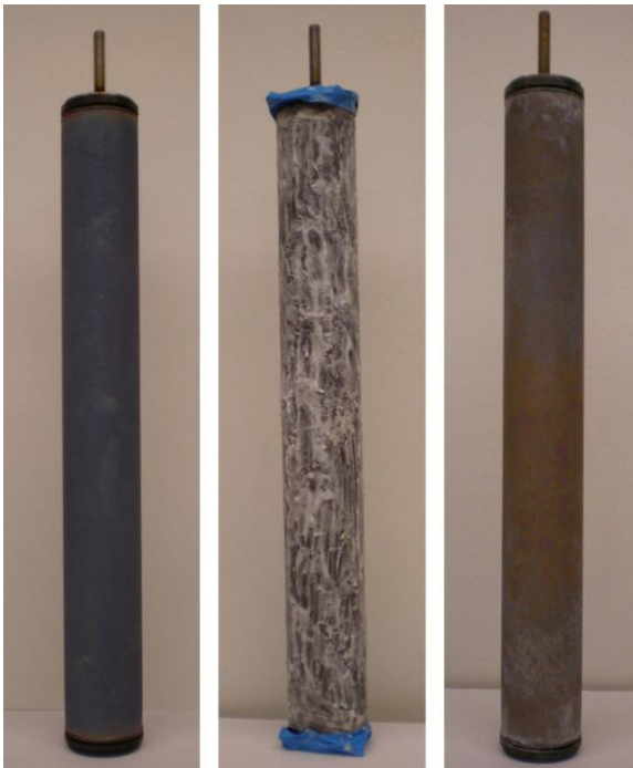
Figure A7. 10 cm diameter by 50 cm length metal tube, before infiltration, after addition of precursor to tube surface, and after firing (from left to right).
