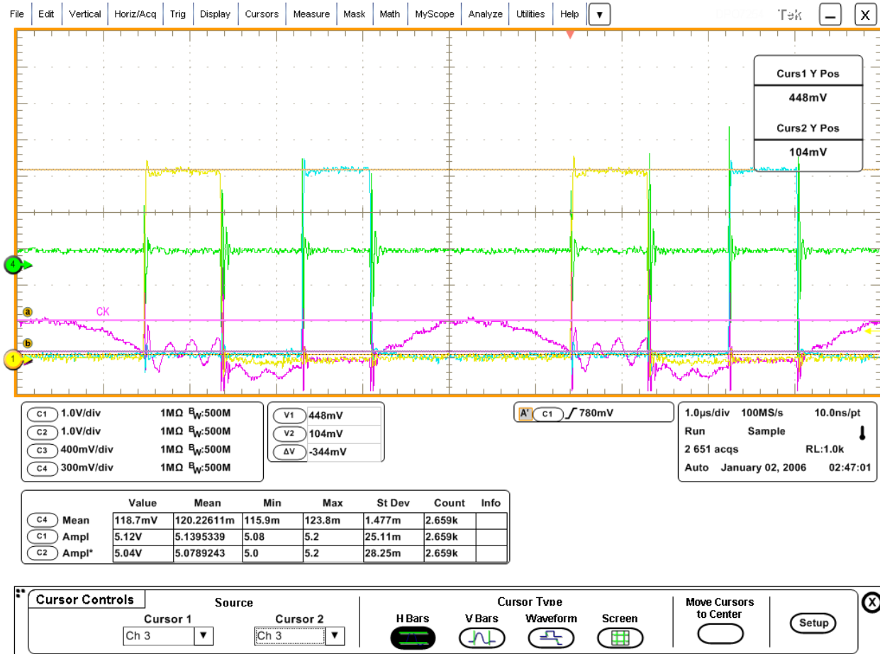
Figure 3.20: Measured output voltage (green), resonator voltage (magenta), and switching signals (yellow and blue) for resonator-based converter with a 100 mV input.
